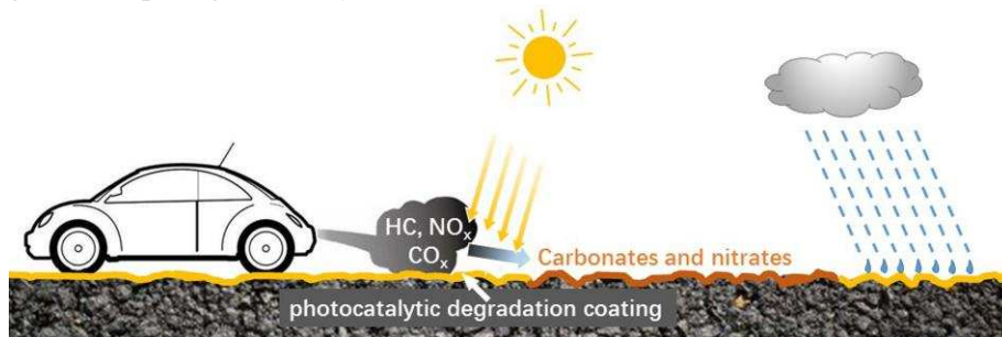
336 337 Fig. 7 Schematic of exhaust gas-decomposing pavement material
