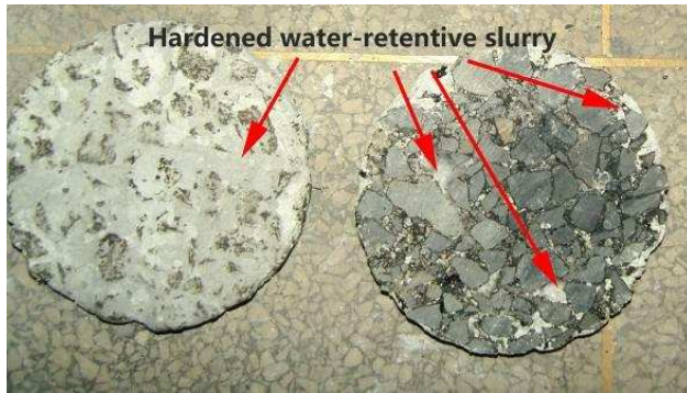
273 Fig. 5 Water-retentive asphalt concrete specimens, surface (left) and cut section (right)
