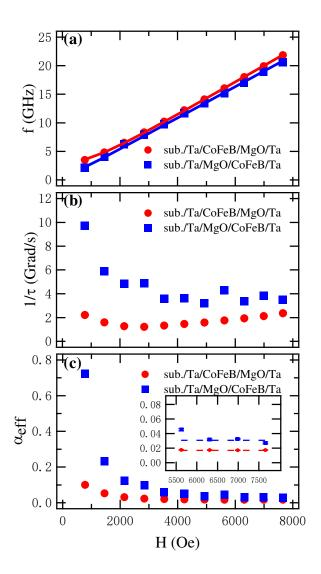
Fig. 4. (Color online) The magnetic field dependence of (a) the precession frequency f and (b) the inverse of relaxation lifetime  $1/\tau$ . The solid lines are the fitting lines. (c) The effective damping constant  $\alpha_{eff}$  as a function of magnetic field. The inset in c) is an enlarged view in the vicinity of H = 6500 Oe and the dotted lines are fitted curves to the experimental data. Error bar denotes the fitting uncertainties.
