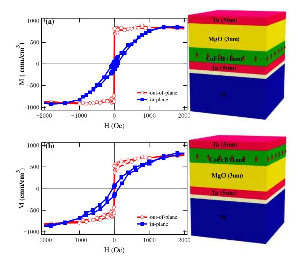
**Fig. 1.** (Color online) The M-H loops measured by VSM for (a) substrate/Ta/CoFeB (1nm)/MgO/Ta and (b) substrate/Ta/MgO/CoFeB (1nm)/Ta. The open circle shows the M-H loop with out-of-plane magnetic field, and the solid square presents the in-plane M-H loop.
