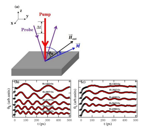
**Fig. 3.** (Color online) (a) Schematic of the TRMOKE measurements. Time-resolved Kerr rotation traces (solid circles) and fitting curves (red lines) for (b) substrate/Ta/CoFeB (1nm)/MgO/Ta and (c) substrate/Ta/MgO/CoFeB (1nm)/Ta films annealed at 300 °C, which were measured by applying various external fields directed at 60° with respect to the film normal direction.
