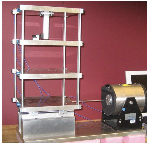
Fig. 3. Image showing setup of the three storey building structure, image reproduced from [53].
