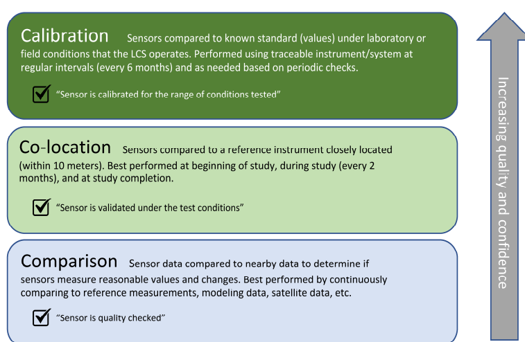
Figure 5. A schematic of typical levels of validation of sensors and instruments
