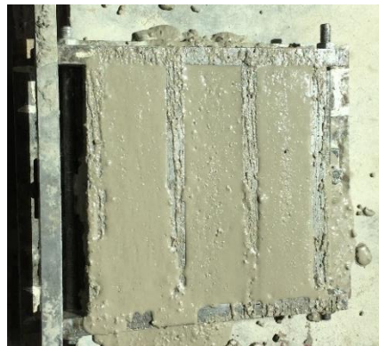
Figure A. 3 Casting RSC flexural prisms
