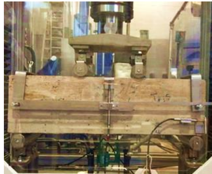
Figure 4.2. Flexural testing of overlaid prism
