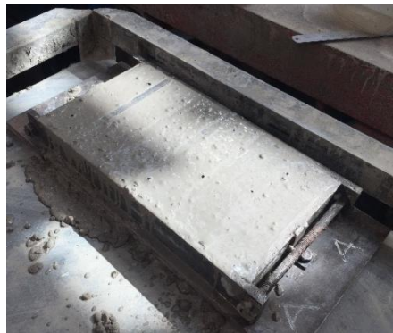
Figure A. 2 Casting CSA flexural prisms
