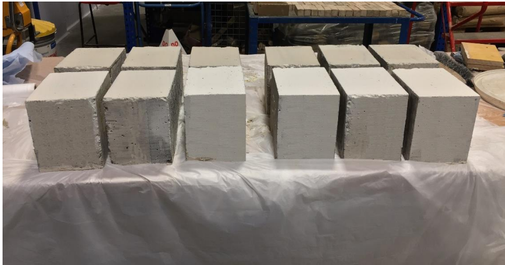
Figure C. 3 Shear samples before testing
