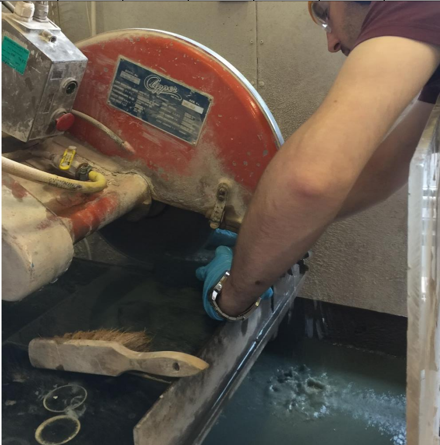
Figure B. 1 The process of slicing moisture transport specimens
