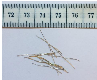
Figure 2.1. Photograph of the RCSF used in this study
