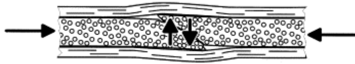
Figure 2-6. Illustration of the explosion effect due to a wedge shaped transverse compressive fracture [37].
