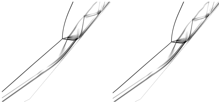
Figure 9: Double cone configuration at 25 - 50 deg. Density gradient. Calorically perfect gas (left), thermally perfect gas (right).
