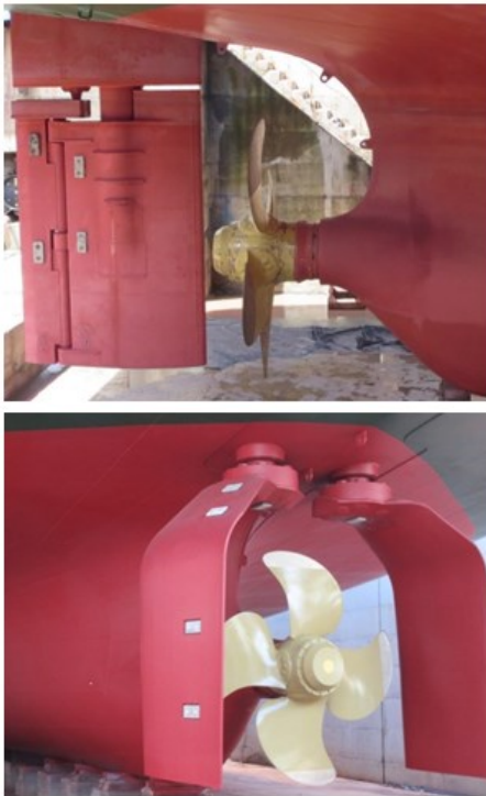
Figure 1. Conventional Flap-Rudder (Top) vs. GATE RUDDER® (Bottom)
