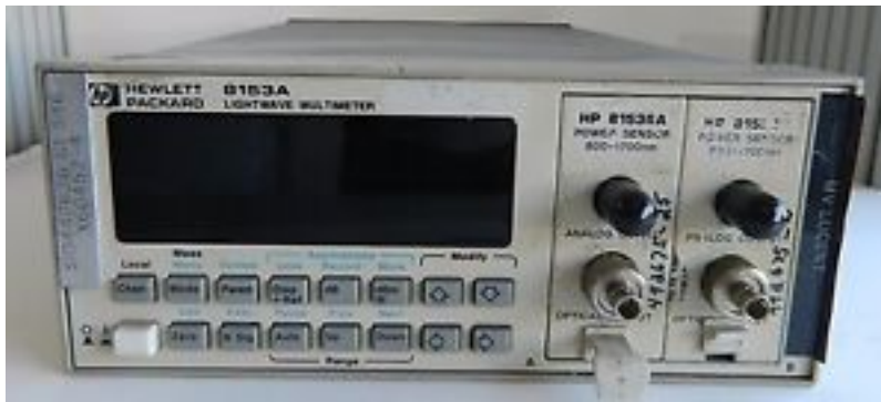
Figure 4-9: HP 8153A Lightwave Multimeter [85].
