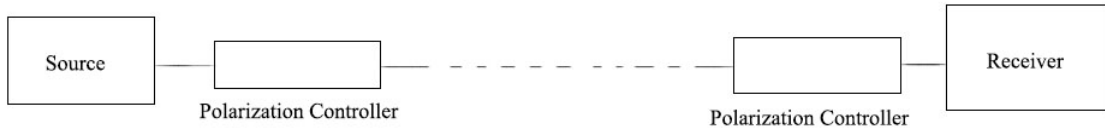
Figure 5-1: Early design of polarization emulator
