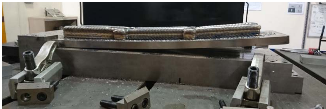
Figure 7 Structural distortion of a WAAM part
