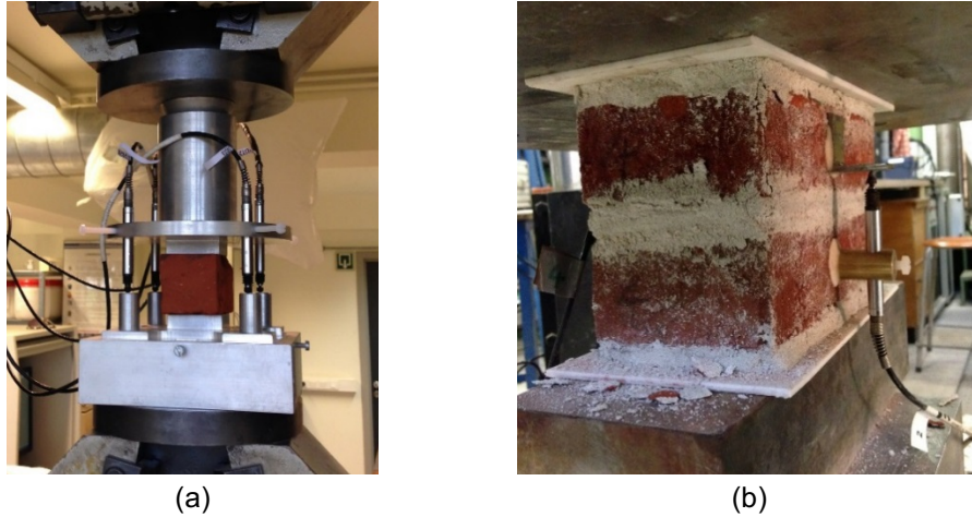
Figure 3. Experimental setup for compression tests on cubes (a) and couplets (b)
