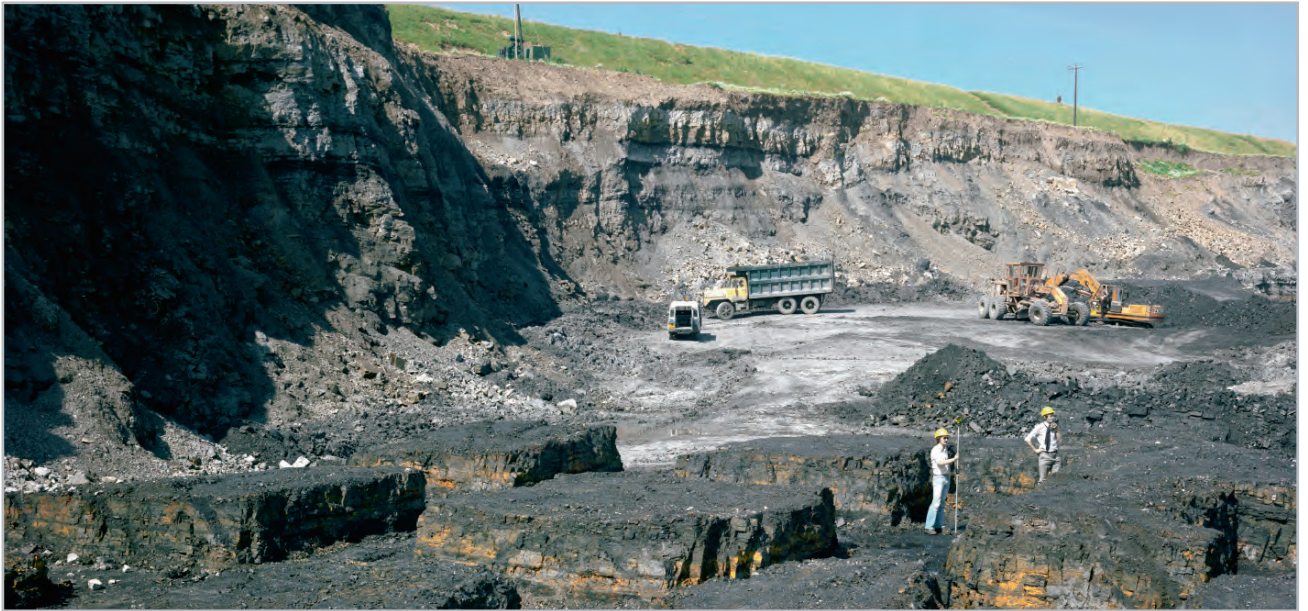
Fig 2: Stoop-and-room (Scottish terminology for pillar-and-room) mine workings subsequently exposed by opencast coal workings at Blindwells, Scotland. Photo number P001520 BGS©UKRI. The image illustrates the connected void space ('rooms') that could be targeted for mine water geothermal projects
