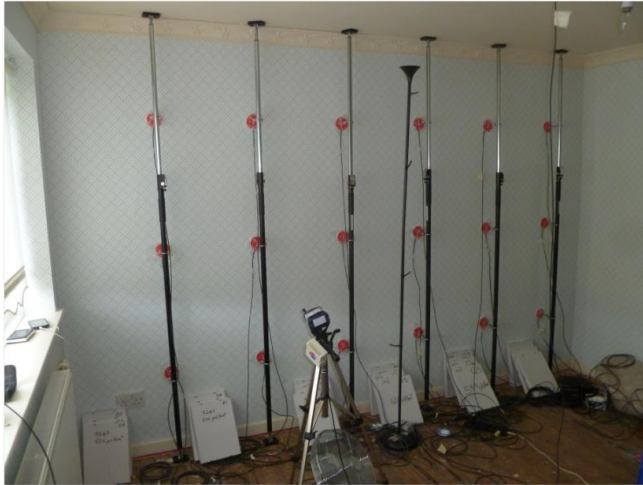
Figure 3.3: Unoccupied homes allowed intensive measurements and a far higher resolution of measurements across the party wall.
