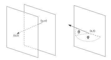
**FIGURE 2** The bi-planar (s, t, u, v) parametrization and the proposed angularly-continuous ( $s, t, \varphi, \theta$ ) parametrization
