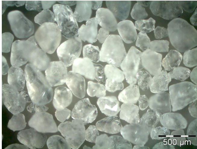
Figure 3: Optical micrograph of the sand particles used in both the dry and water saturated sand slugs.
