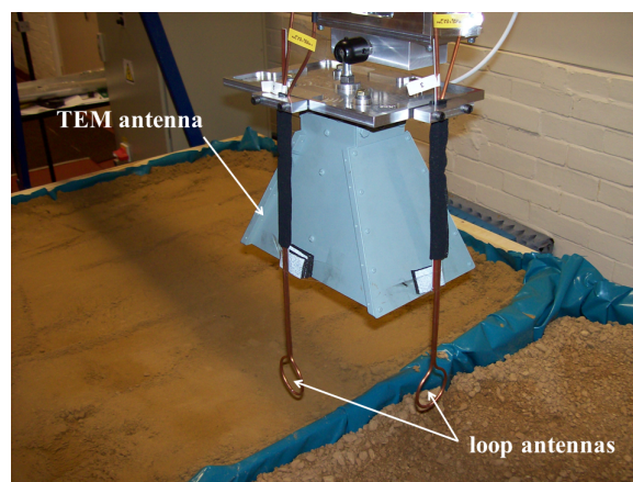
Fig. 1: Photograph of the assembled antenna set-up used in ground penetrating radar experiments. A TEM horn illuminates the ground in vertical (V) polarisation. Two loop antenna are arranged orthogonally to pick up the backscattered VV and VH co-and cross-polarised signals.
