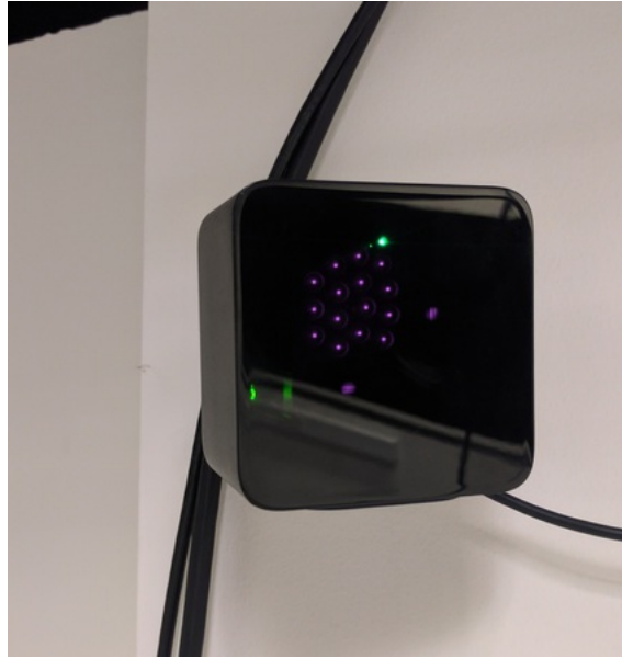
Figure 2.7: One of the base stations used by the VIVE's lighthouse system
