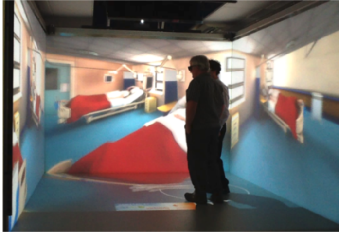
Figure 2.4: The CAVE installation at the University of Keele. Here there are three projection walls but note that CAVES have been built with all four walls, the floor and the ceiling as projection surfaces.
