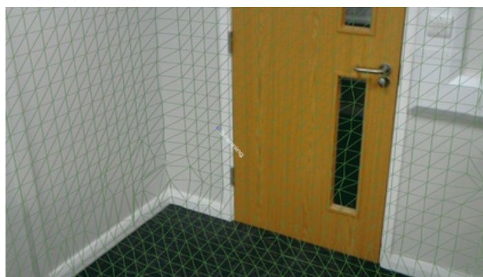
Figure 4.4: A view of the mesh generated by the HoloLens' spatial understanding system, overlaid on to the real world.
