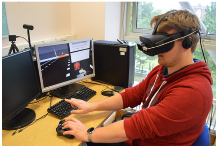
Figure 6.1: Participant using the Oculus Rift with the Leap Motion device attached to the front.
