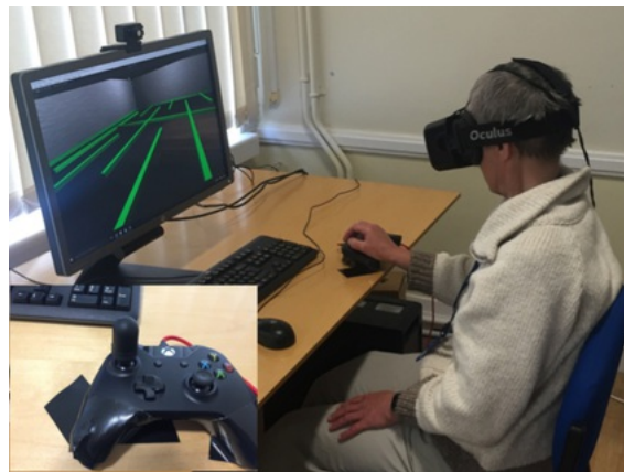
Figure 3.1: The Wheelchair-VR Hardware components consist of the PC, an Oculus Rift DK2 HMD, and an Xbox controller. Insert shows the adapted joystick on the Xbox controller.
