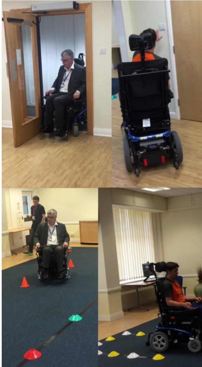
Figure 3.8: The four sections of the timed obstacle course. Top Left - Navigating a doorway. Top Right - Traversing a circular path and using a light switch. Bottom Left - Slalom Course. Bottom Right - Reverse Parking
