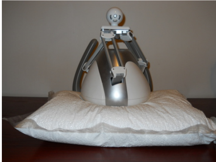
Figure 6.3: The Novint Falcon set up as the wheelchair joystick. It has been rotated by 90 degrees so that the grip interface corresponds to the orientation of the wheelchair joystick. The polystyrene foam bead pillow has been vacuum moulded to the shape of the Falcon to provide stability [22].
