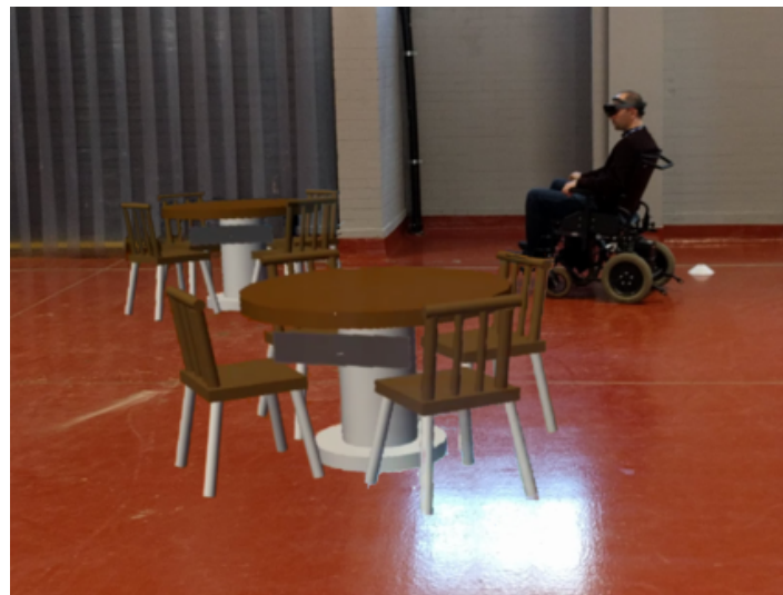
Figure 4.1: The Wheelchair-MR System in use. The user is wearing a Microsoft HoloLens and is driving a powered wheelchair through an empty space in the real world. However, virtual objects (tables and chairs) are present and the user must manoeuvre around them.
