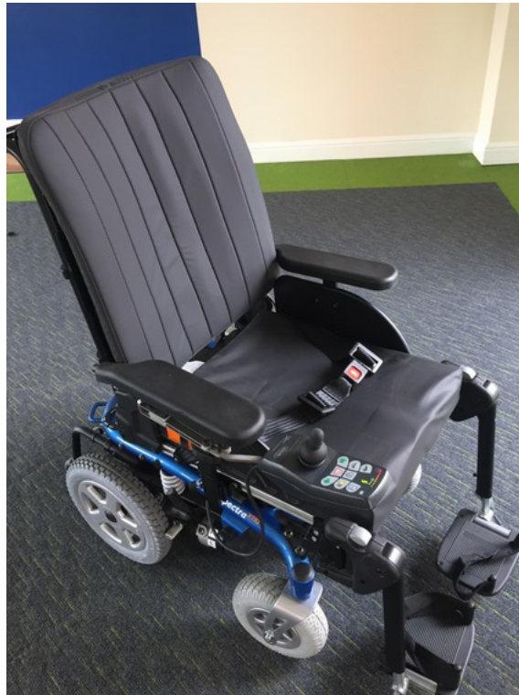
Figure 3.6: The Spectra XTR2 Rear Wheel Drive Wheelchair used in the Validation Study
