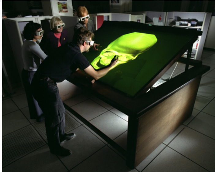
Figure 2.3: Fake Space Immersive Workbench N-239 showing skull for reconstructive surgery studies [5]
