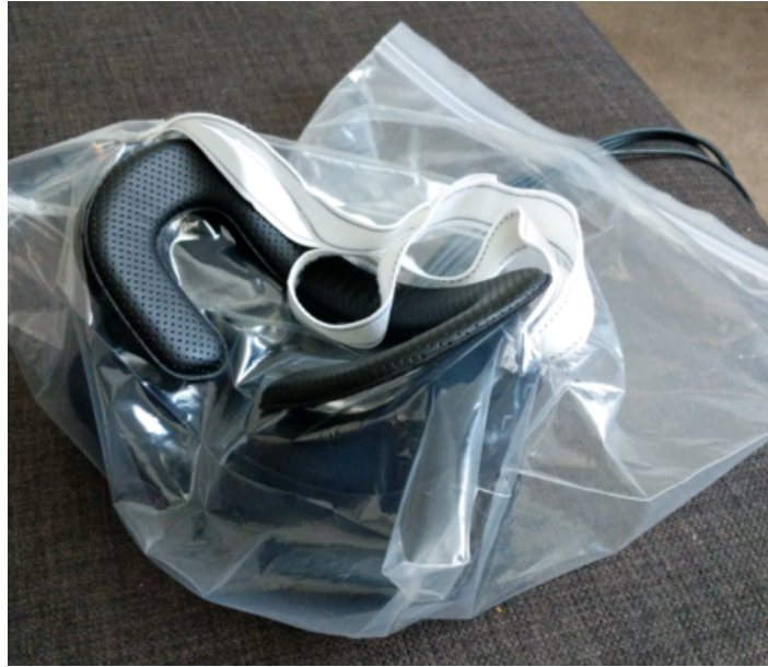
Figure 5.7: The HTC Vive with a disposable head-strap, face-pad and encasing bag.
