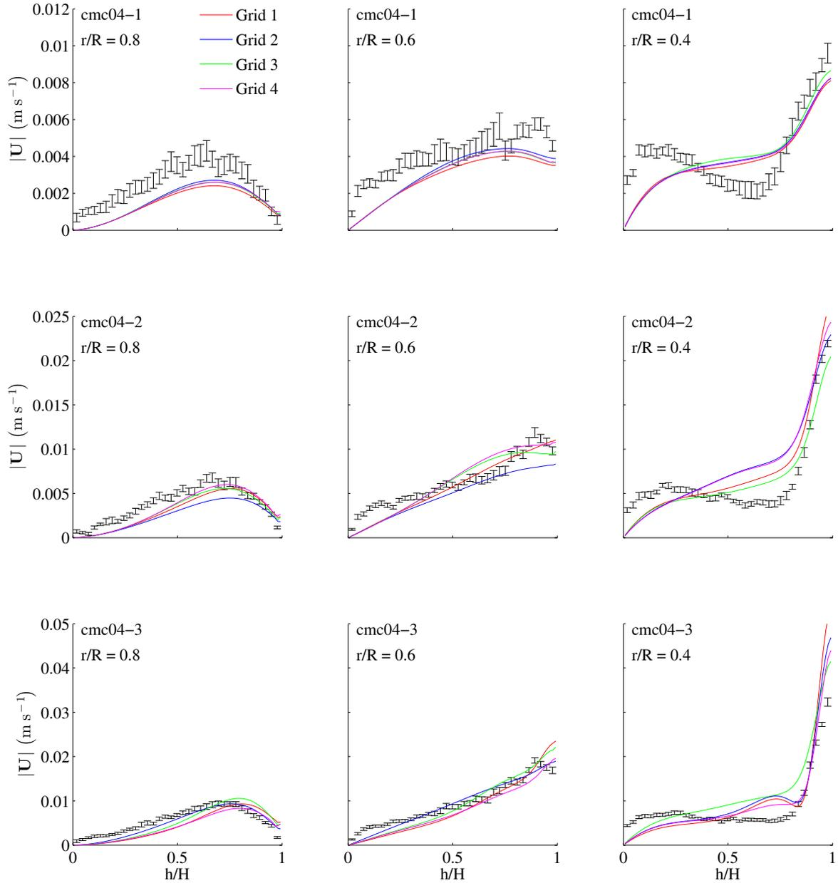
**Figure 8** *CFD-simulated velocity magnitude along a vertical axis against PIV outcome.  $4 \text{ g l}^{-1}$ .*
