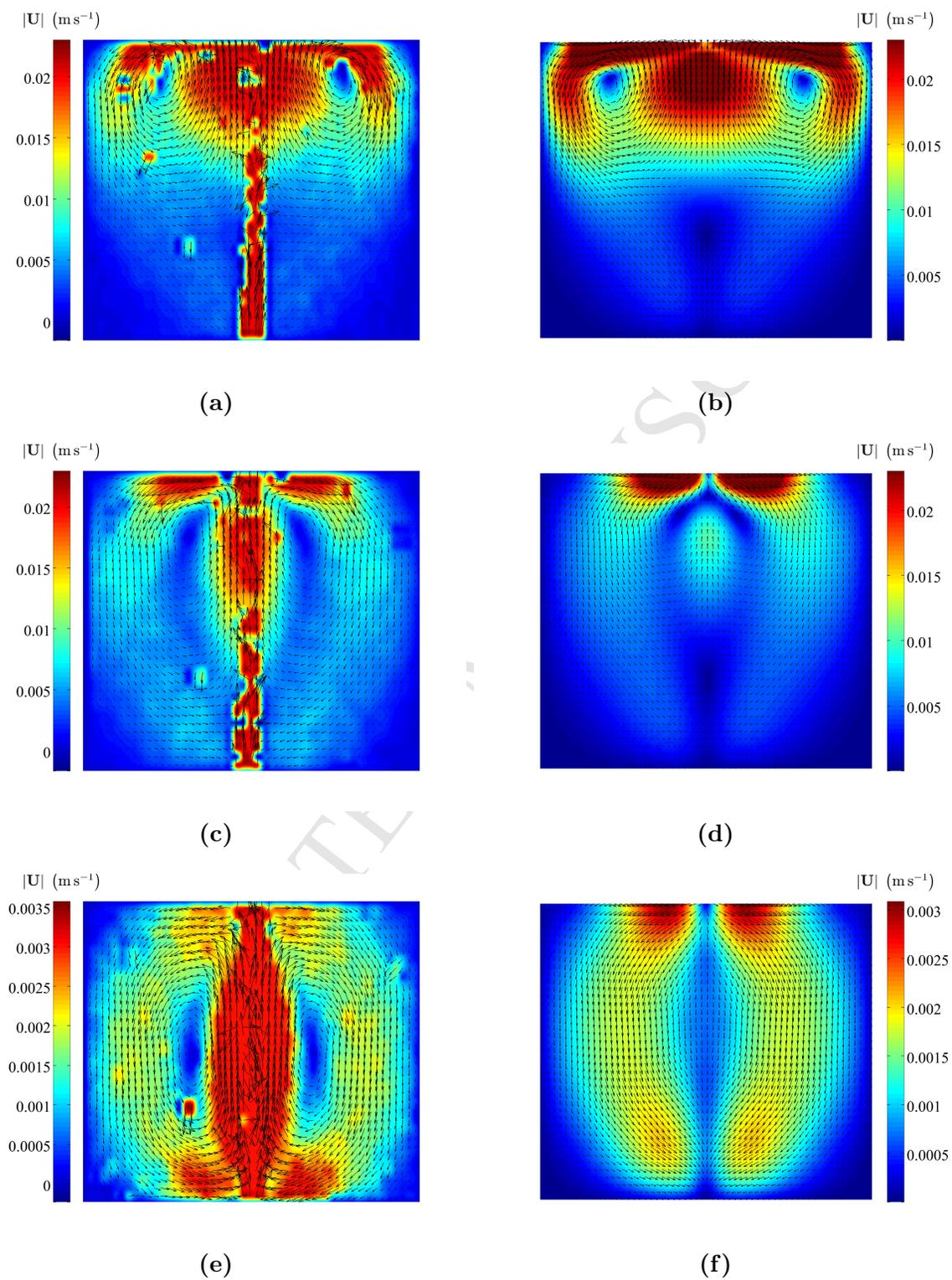
**Figure 5** Projected velocity plots using the Grid 1. *cfd02-2*: (a): PIV outcome, (b): CFD simulation. *cfd04-2*: (c): PIV outcome, (d): CFD simulation. *cfd08-2*: (e): PIV outcome, (f): CFD simulation.
