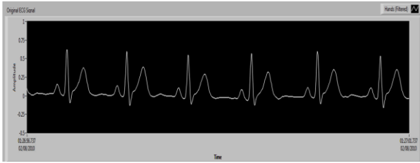
Figure 11: ECG tracing acquired from the output of the hardware's final filtering stage
