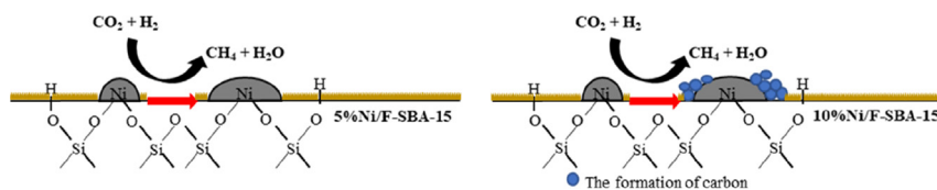
Fig. 7 – Plausible mechanism of Ni/F-SBA-15 towards CO 2 methanation.
