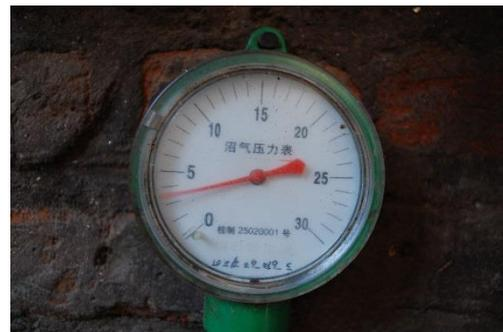
Figure 6: manometer used for the 4x100m<sup>3</sup> digesters. According to the person in charge, pressure can reach about 12 kPa.
