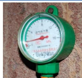
Figure 3: digester's pressure manometer.
