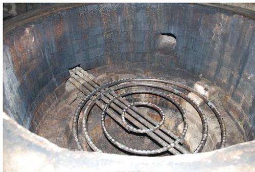
Figure 5: empty 400 L cooker with biogas burner.
