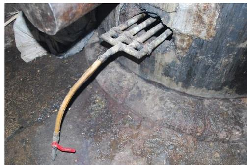
Figure 4: gas inlet for the 400 L cooker.
