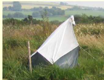
Emergence trap (based on Malaise trap model)
