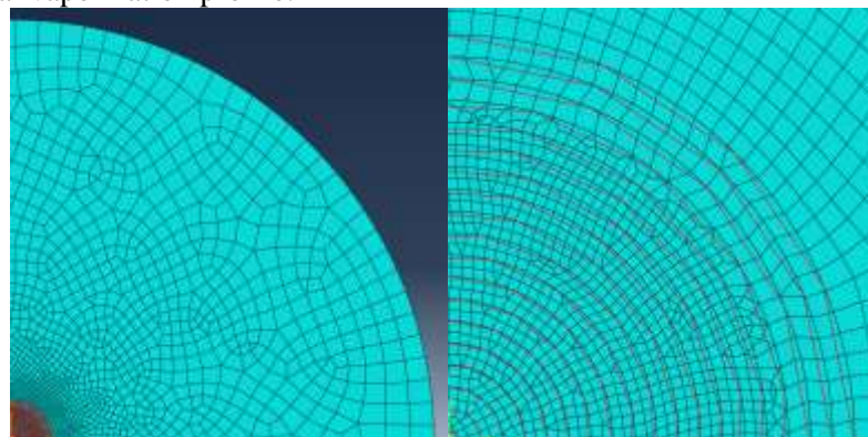
Figure 12 Abaqus GFRP model
