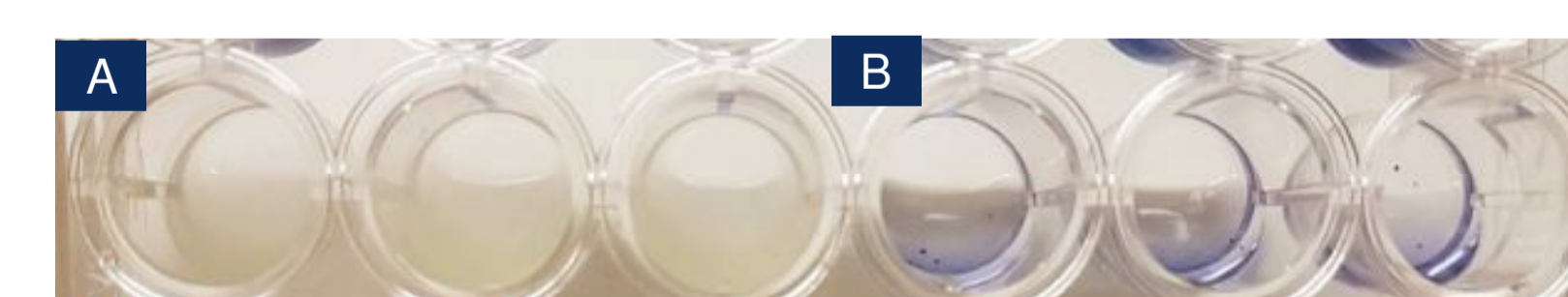
Figure 3 – Decolourisation ability in liquid medium with Blue Supra Everdirect after 24 hours. A – Dye decolourisation with yeast A; B – Control
