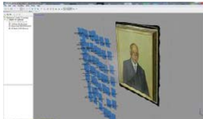
Figure 3 - Screenshot of the photogrammetric project in Agisoft Photoscan® software with the photographs taken in mosaic grid.
