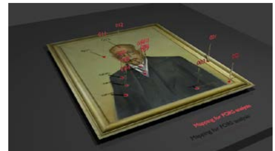
Figure 10 · Virtual scenario made with Blender. The image informs about the location of analysis spots with FORS system.
