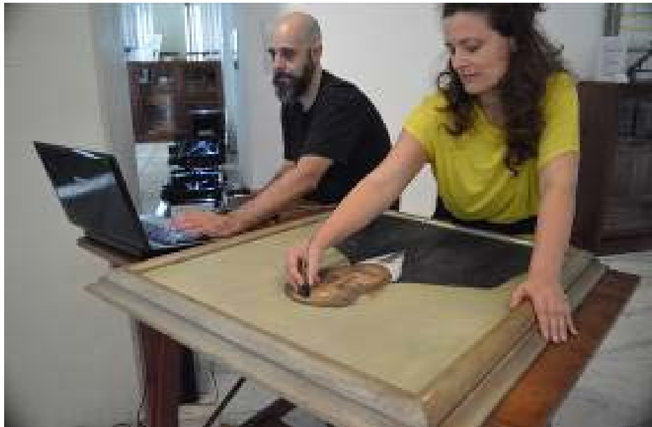
Figure 2 - During the characterization of colour and spectral acquisition with FORS.
