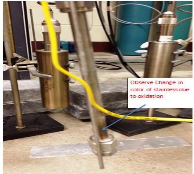
Figure 4-19: Oxidation observed on Stainless Steel
