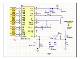
Fig. 3: Voice Chip Circuit
