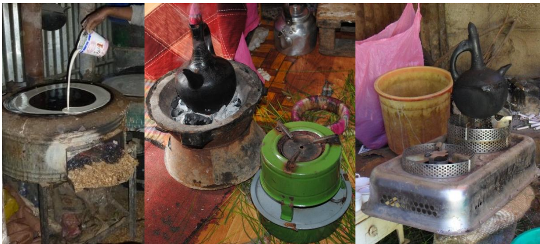
Figure 6.1. Common stoves in Ethiopia. From left to right, a traditional (biomass burning) injera stove, an improved charcoal stove, a kerosene stove and an ethanol stove.
