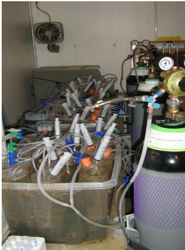
Figure 2.4 Experimental setup for the different aerations conducted in a constant temperature room.
