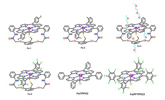
Figure 2:3 Molecular structures of Fe(TPP)Cl, Fe(PFTPP)Cl and basket-handle iron(III) porphrins [39]
