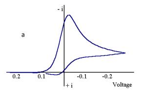
**Figure 1.9 a** The cyclic voltammetry of EC reaction if the chemical reaction is slow. At a low scan rate there is sufficient time for a significant conversion of R to the product and the peak current ratio  $I_p^{\text{back}}/I_p^{\text{forward}}$  is < 1.
