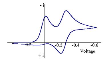
**Figure 1.10** The cyclic voltammetry of ECE reaction. In this illustration the chemical step is fast and two waves are observed for the two E processes
