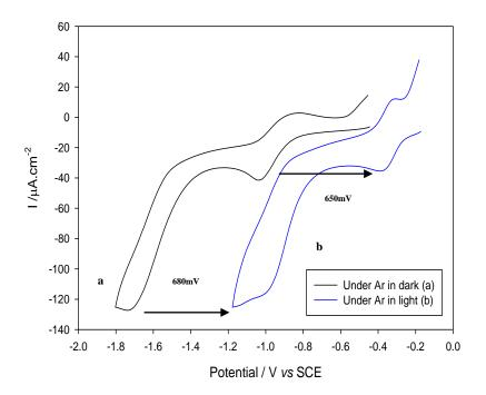
**Figure 3.19** Cyclic voltammograms of **Fe(TPP)Cl** at a p-type H-Si electrode in a solvent mixture (MeCN-5%DMF) containing 0.1M [NBu<sub>4</sub>][BF<sub>4</sub>] at a scan rate of 100mV·s<sup>-1</sup>. (a) in the dark; (b) illuminated by a Krüss halogen fibre optic lamp (90mW·cm<sup>-2</sup>,  $\lambda_{max} = 650$ nm)
