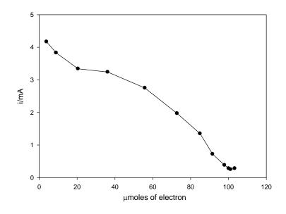
**Figure 3.17** The current *versus* μmoles of electrons passed: 0.2mM **Fe-1** in the presence of CO<sub>2</sub> and 0.274 M CF<sub>3</sub>CH<sub>2</sub>OH in MeCN-5% DMF containing 0.1M [NBu<sub>4</sub>][BF<sub>4</sub>]
