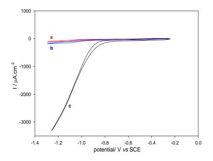
**Figure 3.25** Cyclic voltammograms of **Fe(TPP)Cl** at a p-type H-Si electrode illuminated by a Krüss halogen fibre optic lamp (90mW·cm<sup>-2</sup>,  $\lambda_{max}$  =650nm) in MeCN-5%DMF containing 0.1M [NBu<sub>4</sub>][BF<sub>4</sub>] ,scan rate 100mV·s<sup>-1</sup>. (a) under Ar; (b) in the presence of saturated CO<sub>2</sub>; (c) in the presence of saturated CO<sub>2</sub> and 0.410M CF<sub>3</sub>CH<sub>2</sub>OH
