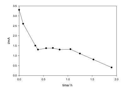
Figure 3.16 Current versus electrolysis time for CO<sub>2</sub> reduction in the presence of Fe(PFTPP)Cl
