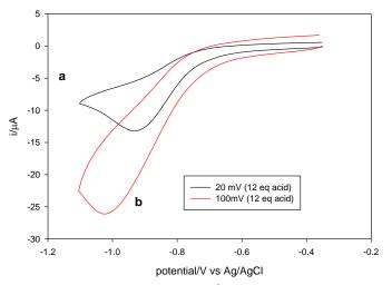
**Figure 4.8** Cyclic voltammetry of 0.5 mM  $[Fe_4S_4(SPh)_4]^{2-}$  in toluene -[Bu4N][BF4], at a vitreous carbon electrode under Ar in the presence 12 equivalents of  $[Hlut]^+$  (a) scan rate  $20mVs^{-1}$ , (b) scan rate  $100mVs^{-1}$
