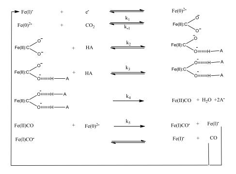
Scheme 3.3 The mechanism of  $CO_2$  reduction in the presence of a catalyst and Bronsted acid as proposed by Saveant and coworkers [17]
