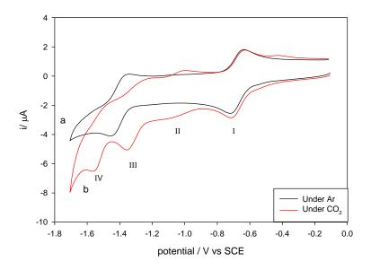
**Figure 3.9** Cyclic voltammetry of 0.2 mM **Fe-1** at a vitreous carbon electrode in MeCN-5% DMF containing 0.1M [NBu<sub>4</sub>][BF<sub>4</sub>], scan rate100mVs<sup>-1</sup>: (a) under Ar; (b) under CO<sub>2</sub> at 1 atmosphere
