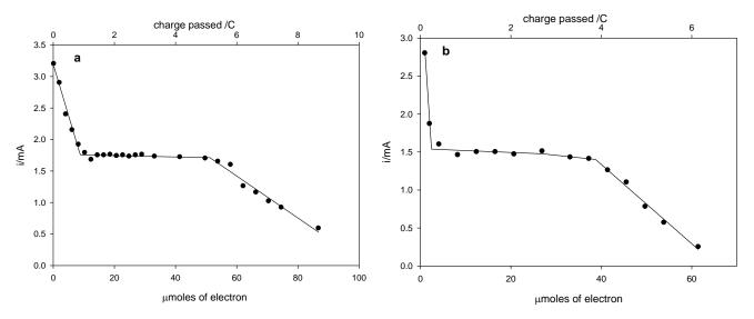
Figure 2.15 Coulometry of cyclooctene epoxidation catalysed by (a) Fe (PFPP)Cl,(b) Fe-4
