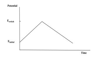
Figure 1.3 The triangular waveform used in cyclic voltammetry
