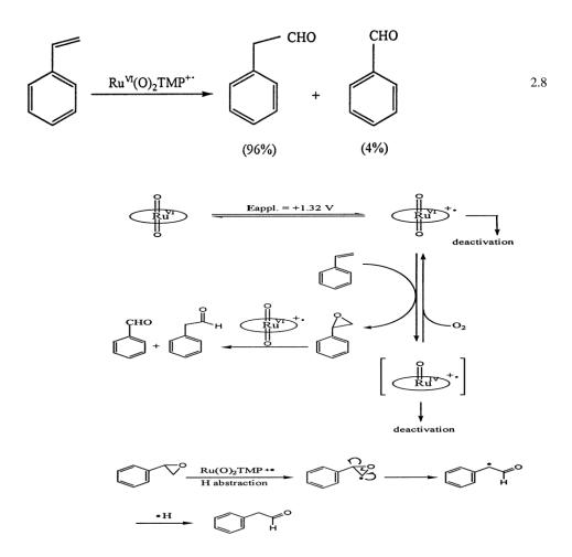
**Scheme 2.2** The reaction mechanism proposed of electrocatalytic oxidation of styrene by a high valent ruthenium porphyrin cation radical [30].
