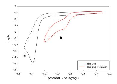
**Figure 4.6** (a) Cyclic voltammetry of 1.5 mM  $[Hlut]^+$  (b) 0.5 mM  $[Fe_4S_4(SPh)_4]^{-2}$  in the presence of 3 eq of  $[Hlut]^+$  in  $[Bu_4N][BF_4]$ -toluene, scan rate100mVs<sup>-1</sup> at a vitreous carbon electrode under Ar
