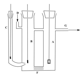
**Figure 1.2** Electrochemical cell A counter electrode, B working electrode, C reference electrode, D, G inlet and outlet taps for purging gas, F a frit for ion exchange.
