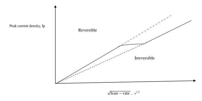
Figure 1.8 The transition of system from reversible to irreversible case with increasing of  $v^{1/2}$ .
