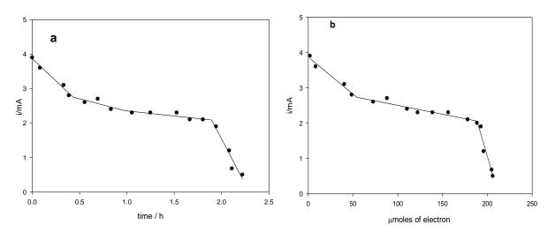
**Figure 3.15** (a) Current *versus* electrolysis time , (b) Current *versus*  $\mu$ moles of electrons for CO<sub>2</sub> reduction in the presence of **Fe(TPP)Cl** . [CF<sub>3</sub>CH<sub>2</sub>OH] = 0.275M (1375 $\mu$ mol)
