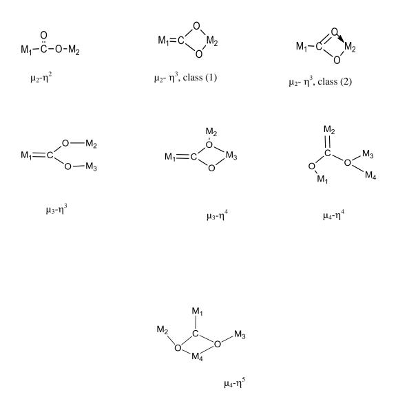
Figure 3.1 Modes of binding for metal-CO $_2$  complexes
