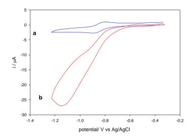
**Figure 4.5** Cyclic voltammetry of 0.5 mM  $[Fe_4S_4(SPh)_4]^{2-}$   $[Bu_4N][BF_4]$ -toluene, scan rate 100mVs<sup>-1</sup> at a vitreous carbon electrode under Ar (a) In the absence of proton source (b) in the presence of 12 eq  $[Hlut]^+$
