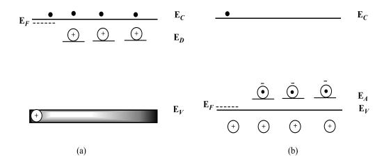
**Figure1.19** Energy band gaps of semiconductor lattices. (a) n-type. (b) p-type.[4] There are other important aspects of semiconductor electrochemistry and photoelectrochemistry which are important to the understanding of electron – transfer at the semiconductor/photoelectrode – solution interface in the presence
