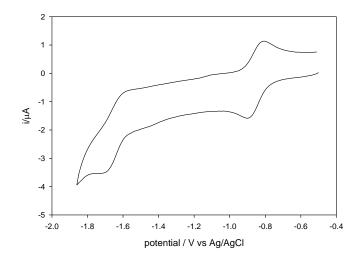
**Figure 4.3** Cyclic voltammetry of 0.5 mM  $[Fe_4S_4(SPh)_4]^{2-}$  in toluene -  $[Bu_4N][BF_4]$ ; scan rate  $100 \text{mVs}^{-1}$ , vitreous carbon electrode under Ar at  $32^{\circ}\text{C}$
