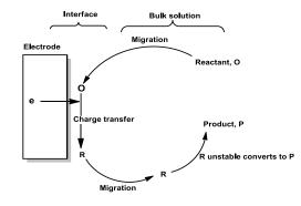
Figure 1.1 Schematic representation of an electrode process.
