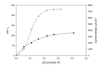
**Figure 3.33** Effect of the acid concentration on  $i_{cat}/i_0$  ratio at a vitreous carbon electrode and at an illuminated p-type H-Si electrode. Solid circles: p-type H-silicon electrode; open circles: vitreous
