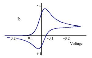
**Figure 1.9 b** At fast scan-rates the time 'window' is sufficiently small so that there is little conversion of R to Y and the peak current ratio  $I_p^{\text{back}}/I_p^{\text{forward}}$  is close to 1.
