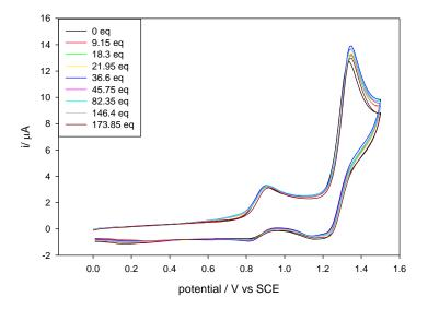
**Figure 2.13** Cyclic voltammograms of **Fe-1** in  $CH_2Cl_2$  containing 0.2 M [Bu<sub>4</sub>N][BF<sub>4</sub>] at room temperature with various adamantane concentrations. Scan rate = 0.1 V s<sup>-1</sup>.
