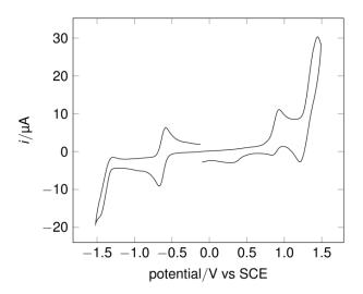
Figure 2.9 Electro-oxidation and reduction of Fe-1 in  $CH_2Cl_2$  containing 0.2M [Bu<sub>4</sub>N][BF<sub>4</sub>] at RT. Scan rate = 0.1V/s.
