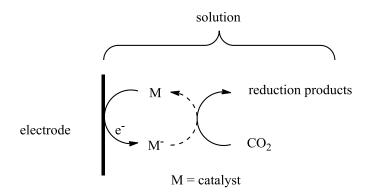
Figure 3.2 General scheme for electrocatalytic reduction of CO<sub>2</sub> [1, 11]
