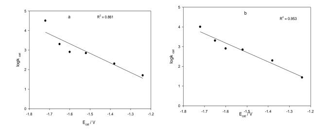
**Figure 3.38** shows the plot of log  $k_{cat}$  for the six complexes *versus*  $E_{cat}$  at vitreous carbon in the presence of saturated CO<sub>2</sub> and 0.18 M CF<sub>3</sub>CH<sub>2</sub>OH. Plot (a) is for 'uncorrected'  $k_{cat}$  data. Plot (b) is that corrected on the assumption that reduced {**Fe(TPP)**} and {**Fe(PFTPP)**} species formed by Cl loss may present two equally accessible faces for catalysis whereas the basket handle thiolate complexes present a single face.
