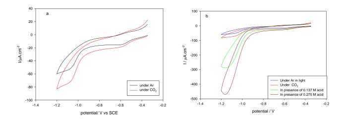
**Figure 3.28** Cyclic voltammetry of 0.2mM **Fe-1** complex in (MeCN-5%DMF) containing 0.1M  $[NBu_4][BF_4]$  *versus* SCE: The scan rate is 100mVs<sup>-1</sup>. (a) Under Ar and CO<sub>2</sub> (b) in the presence of CF<sub>3</sub>CH<sub>2</sub>OH
