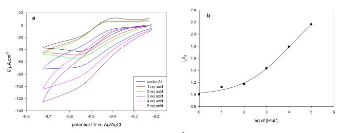
**Figure 4.17** (a) Cyclic voltammograms of  $[Fe_4S_4(SPh)_4]^{2-}$  in the presence of various concentration of [Hlut<sup>+</sup>] at a p-type H-Si electrode illuminated by a Krüss halogen fibre optic lamp (90mW·cm<sup>-2</sup>,  $\lambda_{max} = 650$ nm) toluene-[NBu<sub>4</sub>][BF<sub>4</sub>] at a scan rate of 100mV·s<sup>-1</sup>. (b) The variation of i<sub>cat</sub>/i<sub>0</sub> *versus* concentration of [Hlut<sup>+</sup>]
