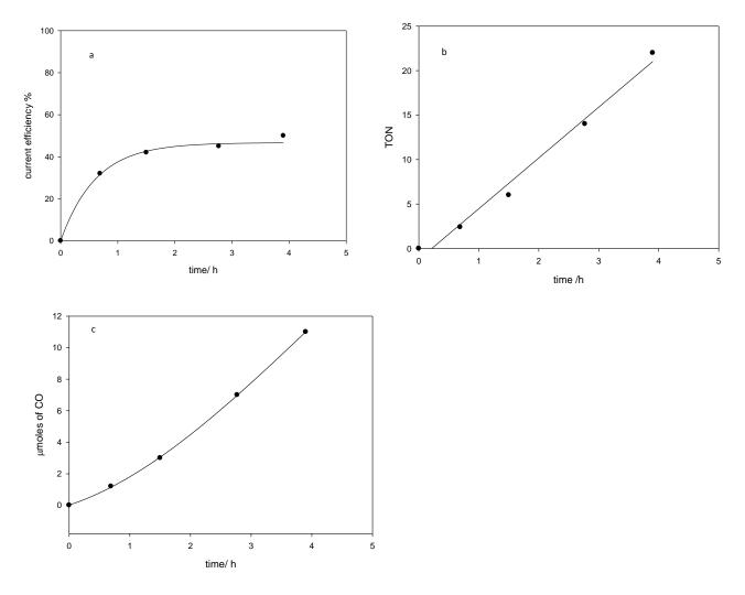
**Figure 3.30** (a) Current efficiency *versus* electrolysis. (b) Turnover number *versus* electrolysis time. (c) µmoles of CO *versus* the electrolysis time
