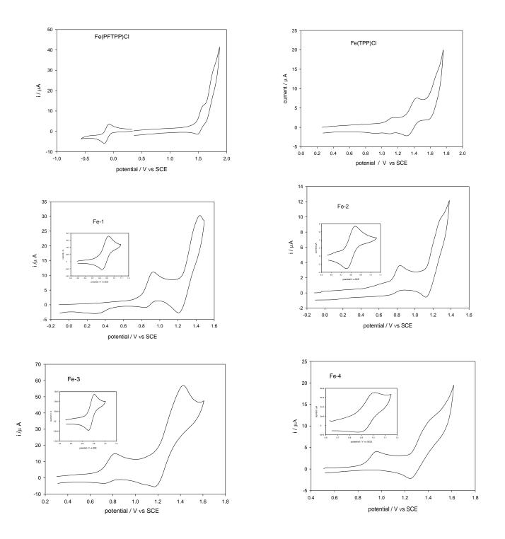
**Figure 2.7** Cyclic voltammograms of **Fe-(1-4**), **Fe(TPP)Cl** and **Fe(PFTPP)Cl** in  $CH_2Cl_2$  containing 0.2M [Bu<sub>4</sub>N[]BF<sub>4</sub>] at RT. Scan rate = 0.1V/s. The inset figures are the quasi-reversible one-electron oxidations (peak 1).
