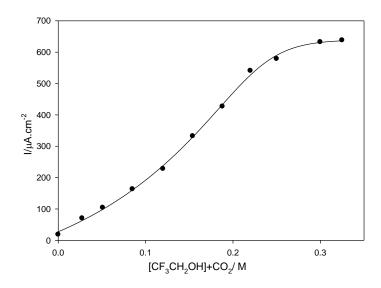
**Figure 3.1.2** Effect of the acid concentration of  $CF_3CH_2OH$  on the peak current for catalysis by **Fe-1** at scan rate 0.1V/s, at room temperature
