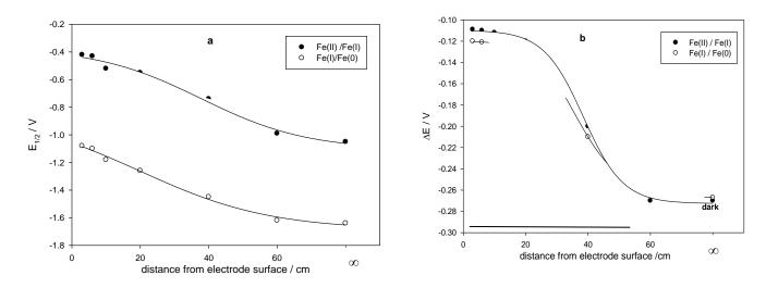
**Figure 3.22** Dependence of (a)  $E_{1/2}$  and (b)  $\Delta E$  values on distance of light source from p-type Si electrode
