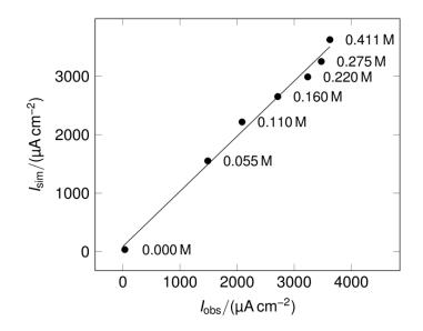
Figure 3.36 Correlation between calculated,  $I_{sim}$ , and experimental,  $I_{obs}$ , current densities at concentrations of  $CF_3CH_2OH$  as labelled in the graph. The simulation is based on the mechanism shown in Scheme 3.6 using the same parameters as given in the text
