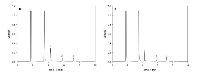
**Figure 2.6** Gas chromatography of cyclooctene epoxidation with PhIO catalysed by (a) **Fe** (**PTPP**) **Cl**, (b) **Fe-1.** 1 is decane, 2 is PhI, 3 is cyclooctene oxide.
