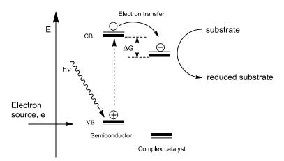
Figure 1.18 Illustration of reduction process on a semiconductor electrode under illumination by light.
