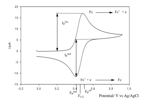
**Figure 1.4** Cyclic voltammogram of a solution of ferrocene in 1.5 mM CH<sub>3</sub>CN/ [NBu<sub>4</sub>][BF<sub>4</sub>] at carbon electrode , scan rate v = 0.025 Vs<sup>-1</sup>.
