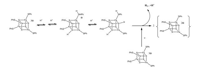
Scheme 4.3: Henderson mechanism of stoichiometric release of dihydrogen release. Adapted from refs [1, 2].
