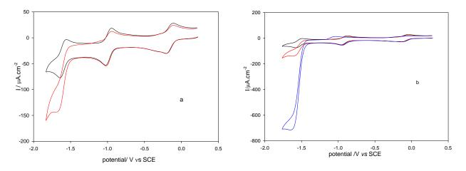
**Figure 3.8** Cyclic voltammetry of 0.2 mM **Fe**(**TPP**)**Cl** at a vitreous carbon electrode in MeCN-5% DMF containing 0.1M [NBu<sub>4</sub>][BF<sub>4</sub>], scan rate100mVs<sup>-1</sup>: (a) under Ar and under CO<sub>2</sub> at 1 atmosphere; (b) in the presence of 0.032 M CF<sub>3</sub>CH<sub>2</sub>OH
