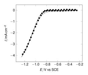
**Figure 3.35** Experimental (solid line) and simulated (closed circles) current density versus potential response for **Fe(TPP)Cl** in the presence of  $CO_2 = 0.25M$  and  $[CF_3CH_2OH] = 0.411M$  at the illuminated p-type Si photocathode
