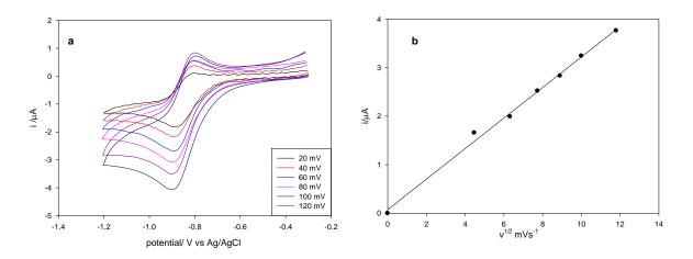
**Figure 4.4** (a) Scan rate dependence of the peak current for the primary reduction process (b) linear dependence of the peak current on the square root of the scan-rate showing the process is diffusion controlled.
