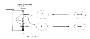
Figure 1.13 The heterogeneous electrocatalysis processes [11].
