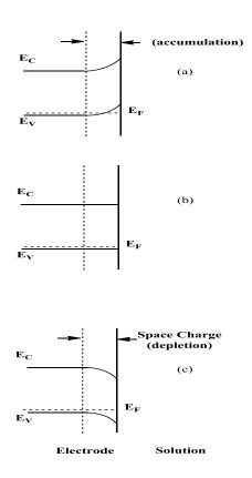
**Figure 1.20** Effect of varying the applied potential (E) on the band edges in the interior of a ptype semiconductor. a)  $E > E_{fb}$  b)  $E = E_{fb}$  c)  $E < E_{fb}$
