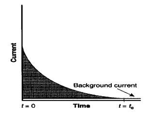
**Figure 1.11** The current change during electrolysis at constant applied potential as the starting material is consumed.
