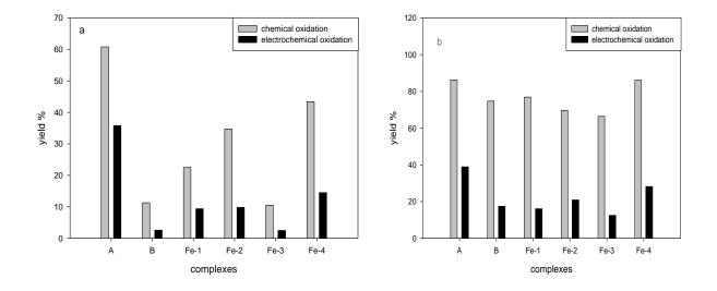
**Figure 2.16** The comparing the yield of (a)1-adamantanol, (b) cyclooctene oxide for chemical and electrochemical oxidation. The yields are based upon iodosobenzene consumed for the chemical oxidation and number of two electron equivalents consumed in the electrochemical oxidation. A = Fe(PFTPP)CI, B = Fe(TPP)CI
