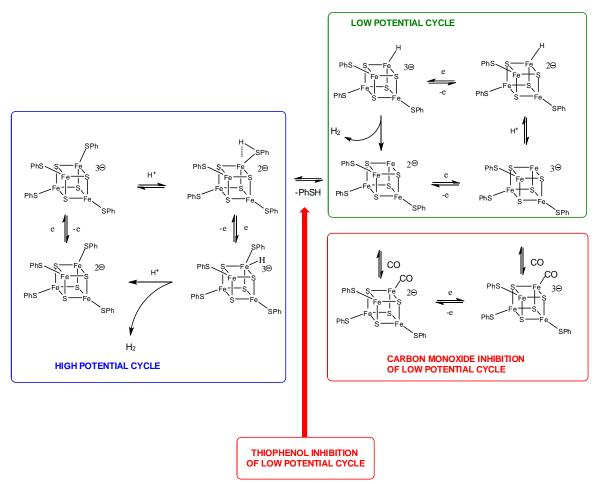
**Scheme 4. 2** Postulated mechanism for hydrogen evolution pathways electrocatalysed by  $[Fe_4S_4(SPh)_4]^{2-}$  and inhibited by CO and by PhSH.
