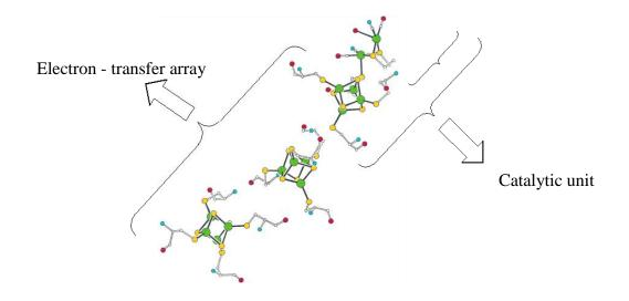
Figure 4.2 Iron sulfur clusters in the [FeFe]-hydrogenases. (X-ray structures : Peters et al 1998,1999 ; Fontecilla-Camps et al 1999) [18]
