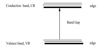
Figure 1.17 The valence and the conduction band in semiconductor
