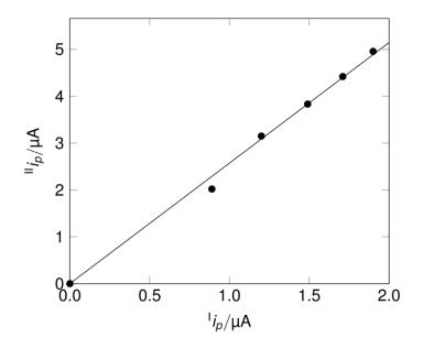
**Figure 2.10** Plots of  ${}^{II}i_{p}^{ox}$  versus  ${}^{I}i_{p}^{ox}$ . Scan rate = 0.1 V s<sup>-1</sup>.
