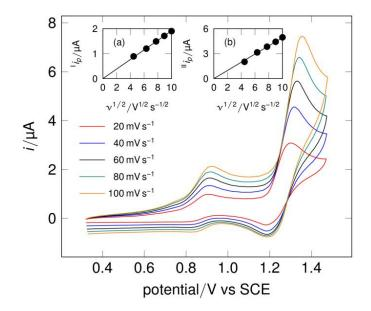
**Figure 2.8** Cyclic voltammograms of **Fe-1** at various scan rate in  $CH_2Cl_2$  containing 0.2 M  $[Bu_4N][BF_4]$ . The inset figures are the plots of  $i_p^{\text{ox}}$  versus  $v^{1/2}$
