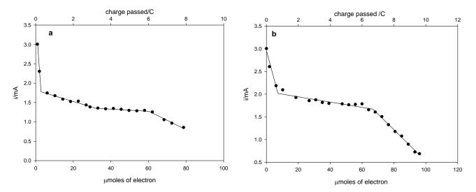
Figure 2.14 Coulometry of adamantane oxidation catalysed by (a). Fe(PFPP)Cl, (b) Fe-2
