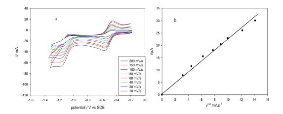
**Figure 3.20** (a) Cyclic voltammograms of 0.22 mM **Fe(TPP)Cl** at illuminated p-type Si at different scan rates in (MeCN-5%DMF) containing 0.1M [NBu<sub>4</sub>][BF<sub>4</sub>] (b) dependence of  $i_p^{red}$  for the Fe(II)/Fe(I) couple on the square root of the scan-rate
