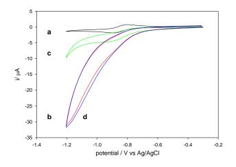
**Figure 4.11** The effect of carbon monoxide on the cyclic voltammetry of  $[Fe_4S_4(SPh)_4]^{2-}$  in the presence of a proton source: (a), black curve, under argon in absence of acid; (b) red curve, in presence of 12 equivalents of acid; (c) green curve, *after* saturating the solution with CO at 1 atmosphere; (d) blue curve, *after* purging CO saturated solution with argon for 6 minutes
