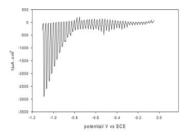
**Figure 3.26** Response of **Fe(TPP)Cl** to chopped light at 2Hz under  $CO_2$  in the presence of 0.275 M CF<sub>3</sub>CH<sub>2</sub>OH, scan rate 50 mVs<sup>-1</sup>
