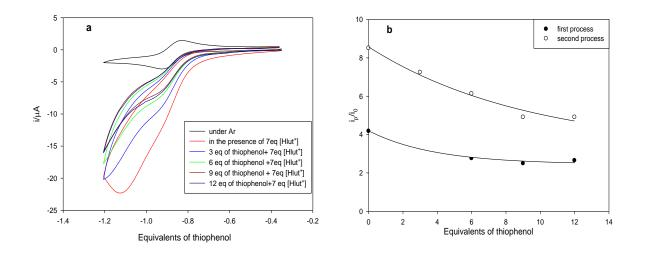
**Figure 4.13** (a) The effect of the addition of thiophenol on proton reduction electrocatalysed  $[Fe_4S_4(SPh)_4]^{2-}$ . (b) The  $i_{cat}/i_0$  ratio at a vitreous carbon electrode( first and second process)
