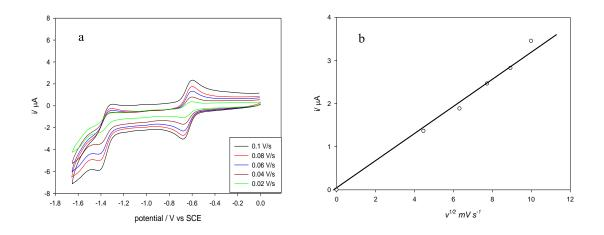
**Figure 3.6** (a) Cyclic voltammograms of 0.22 mM **Fe-1** at carbon electrode, at different scanrates in (MeCN-5%DMF) containing 0.1M [NBu<sub>4</sub>][BF<sub>4</sub>]. (b) Plot of  $i_p^{red}$  for the Fe(II)/Fe(I) couple versus the square-root of the scan-rate ( third reduction at -1.82 V)
