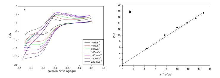
**Figure 4.16** (a) Cyclic voltammograms of 0.5mM  $[Fe_4S_4(SPh)_4]^{2-}$  at p-type Si electrode (first reduction) at different scan rates in toluene- $[Bu_4N][BF_4]$ . (b) Plot of  $i_p^{red}$  versus  $v^{1/2}$
