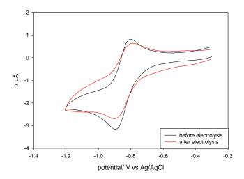
Figure 4.10 Cyclic voltammetry of  $[Fe_4S_4(SPh)_4]^{2-}$  before and after electrolysis
