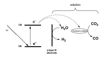
**Scheme3.5** Heterogeneous catalysis role of p-type Si for  $H_2$  reduction from  $H_2O$  and the Feporphyrin role as  $CO_2$  reduction catalysts. Adapted from ref. [38].
