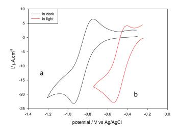
**Figure 4.15** Cyclic voltammograms of  $[Fe_4S_4(SPh)_4]^{2-}$  at a p-type H-Si electrode in toluene-[NBu<sub>4</sub>][BF<sub>4</sub>], scan rate 100mV·s<sup>-1</sup>. (a) In the dark; (b) illuminated by a Krüss halogen fibre optic lamp (90mW·cm<sup>2</sup>,  $\lambda_{max} = 650$ nm)
