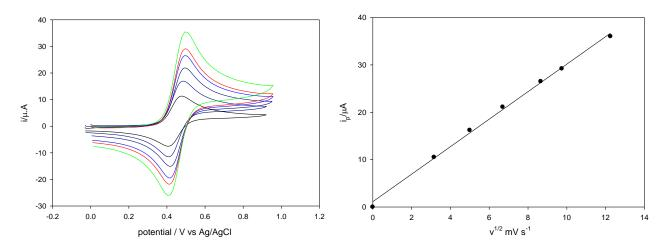
**Figure 1.5** Cyclic voltammograms obtained for 1.5 mM ferrocene in CH<sub>3</sub>CN at a glassy carbon electrode (0.072 cm<sup>2</sup>) at scan rates of : 0.01, 0.025, 0.045, 0.075, 0.095, and 0.15 V/s. (b) The dependence of square root of the scan-rate ( $v^{1/2}$ ) on the peak current for oxidation of ferrocene.
