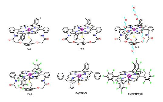
**Figure 3.4** Molecular structures of **Fe(TPP)Cl**, **Fe(PFTPP)Cl** and basket-handle iron(III) porphrins together with their abbreviations used in the text
