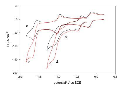
**Figure 3.24** Cyclic voltammetry of 0.2 mM **Fe(TTP)Cl** complex in (MeCN-5%DMF) containing 0.1M [NBu<sub>4</sub>][BF<sub>4</sub>] scan rate100mVs<sup>-1</sup>. Black curves: (a) at a vitreous carbon electrode under Ar (b) at illuminated 1-10 ohm cm<sup>-1</sup> p-type Si electrode under Ar. Red curves: (c) at a vitreous carbon electrode under CO<sub>2</sub> (d) at an illuminated 1-10 ohm cm<sup>-1</sup> p-type Si electrode under CO<sub>2</sub>
