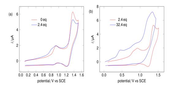
**Figure 2.11** Cyclic voltammograms of **Fe-1** in  $CH_2Cl_2$  containing 0.2 M [Bu<sub>4</sub>N][BF<sub>4</sub>] at room temperature with added [Bu<sub>4</sub>N][OH]. Scan rate = 0.1 V s<sup>-1</sup>
