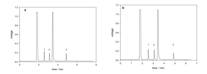
**Figure 2.4** Gas chromatography of adamantane oxidation with PhIO catalysed by (a) **Fe** (**PFPP)Cl**,(b) **Fe-4.** 1 is PhBr, 2 is PhI, 3 is 1-adamantanol.
