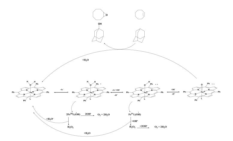
Scheme 2.5 Proposed mechanism of electrocatalytic oxidation of hydrocarbon.
