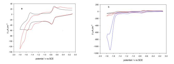
**Figure 3.13** Cyclic voltammetry of **Fe-2** (0.2 mM) at a vitreous carbon electrode in MeCN-5%DMF containing 0.1M [NBu<sub>4</sub>][BF<sub>4</sub>]; scan rate100mVs<sup>-1</sup>, (a) under CO<sub>2</sub>, (b) in the presence of 0.21 M CF<sub>3</sub>CH<sub>2</sub>OH
