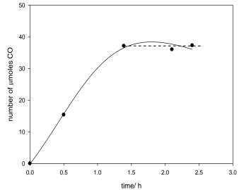
**Figure 3.18** CO yield *versus* electrolysis time, 0.1mM **Fe-1**, 0.274 M CF<sub>3</sub>CH<sub>2</sub>OH and saturated  $CO_2$  (*ca* 0.27M) in a MeCN-5%DMF containing 0.1M [NBu<sub>4</sub>][BF<sub>4</sub>]
