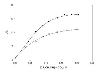
**Figure 3.37** Effect of the acid concentration on  $icat/i_0$  ratio at a vitreous carbon electrode and an illuminated p-type H-Si electrode. Solid circles: carbon electrode; open circles p-type Si electrode
