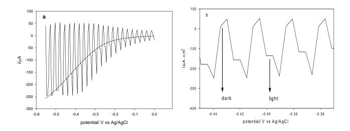
**Figure 4.18** Response of  $[Fe_4S_4(SPh)_4]^{2-}$  to chopped light at 2Hz the presence of 12 eq  $[Hlut^+]$ , scan rate 50 mVs<sup>-1</sup>. (a) Response from -0.0 to- 0.6 V. (b) An expanded region of this response in the range - 0.3 to -0.5 V *versus* Ag/AgCl
