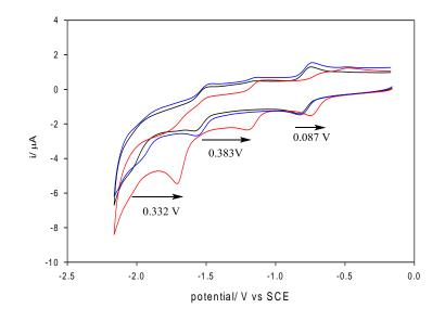
**Figure 3.14** Cyclic voltammetry of 0.2 mM **Fe-3** in (MeCN-5%DMF) containing 0.1M  $[NBu_4][BF_4]$ , scan rate100 mVs<sup>-1</sup> at a vitreous carbon electrode under Ar , in the presence of proton source and the presence of potassium *tertiary* butoxide
