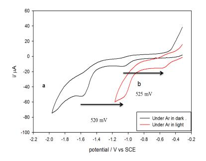
**Figure 3.23** The cyclic voltammetry 0.1mM **Fe-1** in (MeCN-5%DMF) containing 0.1M [NBu<sub>4</sub>][BF<sub>4</sub>] of 0.1 mM **Fe-1** (a) in the dark under Ar (b) illuminated by light
