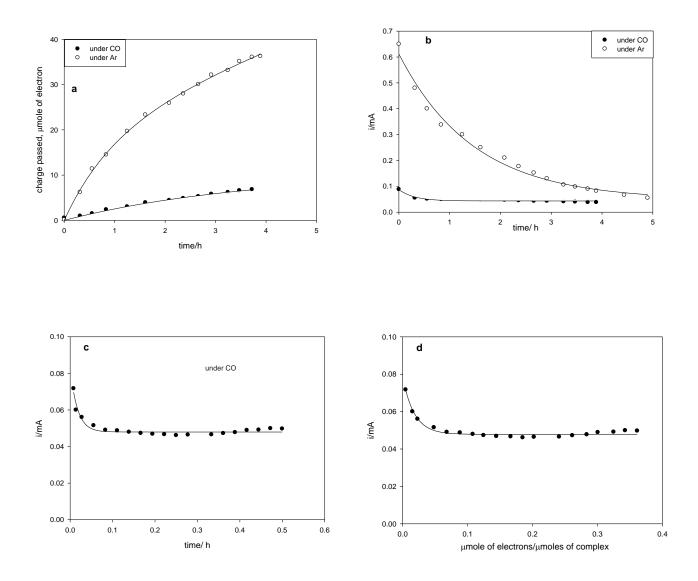
**Figure 4.12** (a) Charge passed *versus* electrolysis time, (b) current *versus* electrolysis time, (c) an expansion of the current – time course in this initial phase.(d) the corresponding plot of current *versus* charge passed (moles of electrons/moles of cluster). Electrolysis of 0.5 mM  $[Fe_4S_4(SPh)_4]^{2^-}$  in  $[Bu_4N][BF_4]$ -toluene in the presence of 12eq [Hlut<sup>+</sup>] on a vitreous carbon electrode (2cm<sup>2</sup>) under Ar and CO at -0.9 V vs Ag/AgCl.
