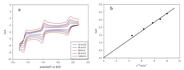
**Figure 3.5** (a) Cyclic voltammograms of 0.22 mM **Fe(TPP)Cl** at carbon electrode, at different scan-rates in (MeCN-5%DMF) containing 0.1M [NBu<sub>4</sub>][BF<sub>4</sub>]. (b) Plot of  $i_p^{red}$  for the Fe(II)/Fe(I) couple versus the square-root of the scan-rate
