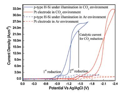
**Figure 3.3** Photo-electrocatalytic CO<sub>2</sub> reduction with Re (4,4-*t*Bu<sub>2</sub>bpy)(CO)<sub>3</sub>Cl on a *p*-type Si electrode. Reproduced from reference [26]
