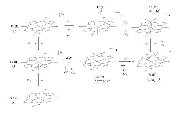
**Scheme 3.6** Proposed pathway for photoelectrocatalysis of  $CO_2$  reduction to CO. Values of  $E^{\circ}$ 's, equilibrium  $K_n$  constants and rate constants  $k_n$  together with other experimental and fitted parameters used in digital simulations are given below
