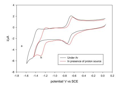
**Figure 3.10** Cyclic voltammetry of 0.2 mM **Fe-1** at a vitreous carbon electrode in MeCN-5% DMF containing 0.1M [NBu<sub>4</sub>][BF<sub>4</sub>], scan rate100mVs<sup>-1</sup>: (a) under Ar ; (b) in the presence of  $CF_3CH_2OH$  at 0.274M
