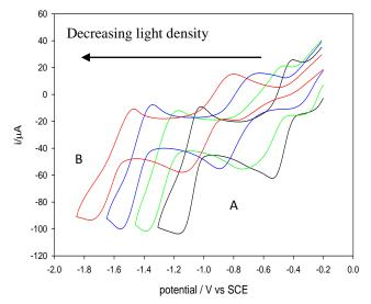
**Figure 3.21** The effect of light intensity on the cyclic voltammetry of 0.2 mM **Fe(TPP)Cl** at p-type Si, in (MeCN-5%DMF) containing 0.1M [NBu<sub>4</sub>][BF<sub>4</sub>]
