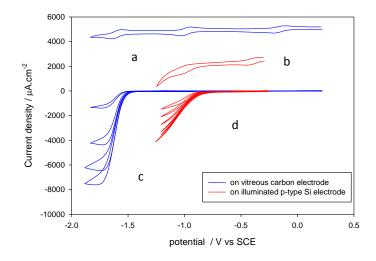
**Figure 3.32** Cyclic voltammetry of **Fe(TPP)Cl** (0.22mM) in (MeCN-5%DMF) containing 0.1M [NBu<sub>4</sub>][BF<sub>4</sub>], Rt. Scan rate 100 mVs<sup>-1</sup>. (a) at vitreous carbon electrode under Ar (b) at illuminated p-type Si electrode under Ar (c) at vitreous carbon electrode under 1 atm of CO<sub>2</sub> in presence of 0.055M, 0.11M, 0.16M, and 0.22M CF<sub>3</sub>CH<sub>2</sub>OH (d) at illuminated p-type Si electrode under same condition as in (c)
