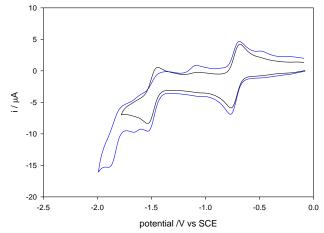
**Figure 3.7** Cyclic voltammetry of 0.22 M **Fe-2** at a at a vitreous carbon electrode in MeCN-5% DMF containing 0.1M [NBu<sub>4</sub>][BF<sub>4</sub>], scan rate100mVs<sup>-1</sup> under Ar
