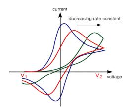
Figure 1.7 Schematic representation of a quasi-reversible system
