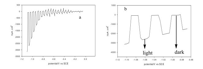
**Figure 2.27** Response of **Fe(TPP)Cl** to chopped light at 1Hz under  $CO_2$  in the presence of 0.275 M CF<sub>3</sub>CH<sub>2</sub>OH, scan rate 50 mVs<sup>-1</sup>.(a) Response from -0.0 to 1.1V.(b) An expanded region of this response in the range - 0.98 and -1.1 V versus SCE
