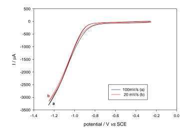
**Figure 3. 34** Cyclic voltammograms of A at a p-type H-Si electrode illuminated by a Krüss halogen fibre optic lamp (90mW cm<sup>-2</sup>,  $\lambda_{max}$  =650nm) in a solvent mixture (MeCN-5%DMF) containing 0.1M [NBu<sub>4</sub>][BF<sub>4</sub>] in the presence of saturated CO<sub>2</sub> and 0.411 M CF<sub>3</sub>CH<sub>2</sub>OH : (a) scan rate = 100mV s<sup>-1</sup>, (b) scan rate = 20mV s<sup>-1</sup>
