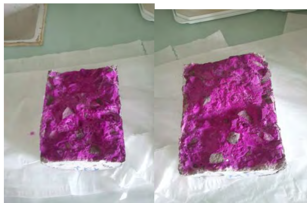
Figure B. 7: Concrete specimen for control of carbonation. Carbonation ingress tested with phenolphthalein after one month (right) and two months (left). Violet colour indicates that the specimen is not carbonated.
