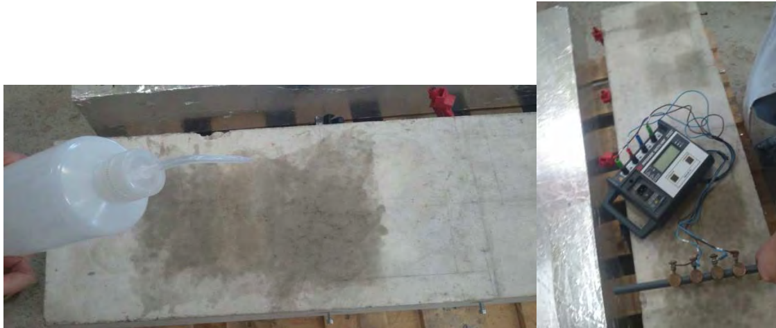
Figure VI. 15: Measurement of concrete resistivity on the slabs via the technique of Wenner. A slight humidification of the concrete surface is required in order to eliminate problems of resistance of contact.
