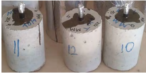
Figure VI. 8: Cylindrical reinforced concrete specimen, used for the Tafel constant measurements
