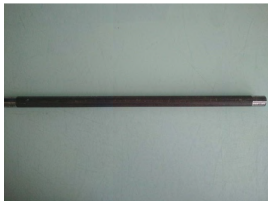
Figure VI. 6: Steel rebar after cleaning it with acetone and ethanol to remove the grease and before embedding it into the concrete. No mechanical treatment was carried out.
