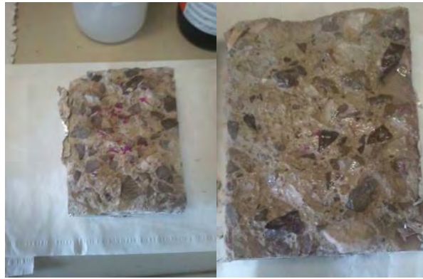
Figure B. 6: Concrete specimen for control of carbonation. Controlling the ingress of carbonation with phenolphthalein after one month (right) and two months (left).
