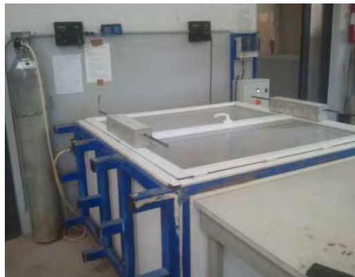
Figure B. 4: Chamber of accelerated carbonation (50%CO 2 , 60%.RH)
