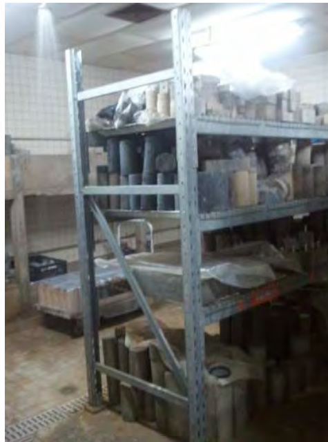
Figure B. 2:24h curing of the concrete specimens in a chamber of fixed temperature (20°C) and relative humidity (95°C).
