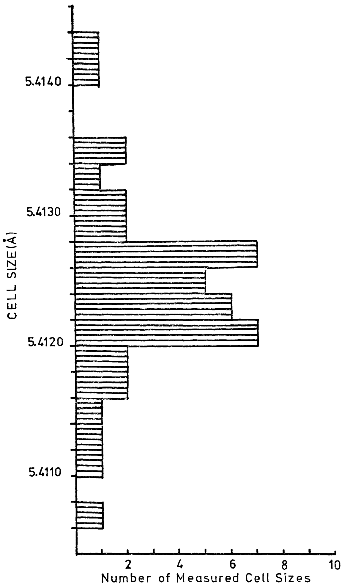
Fig5.9.2 Frequency Diagram of Cell Sizes Measured on Sphalerite from the Bulancak Area
