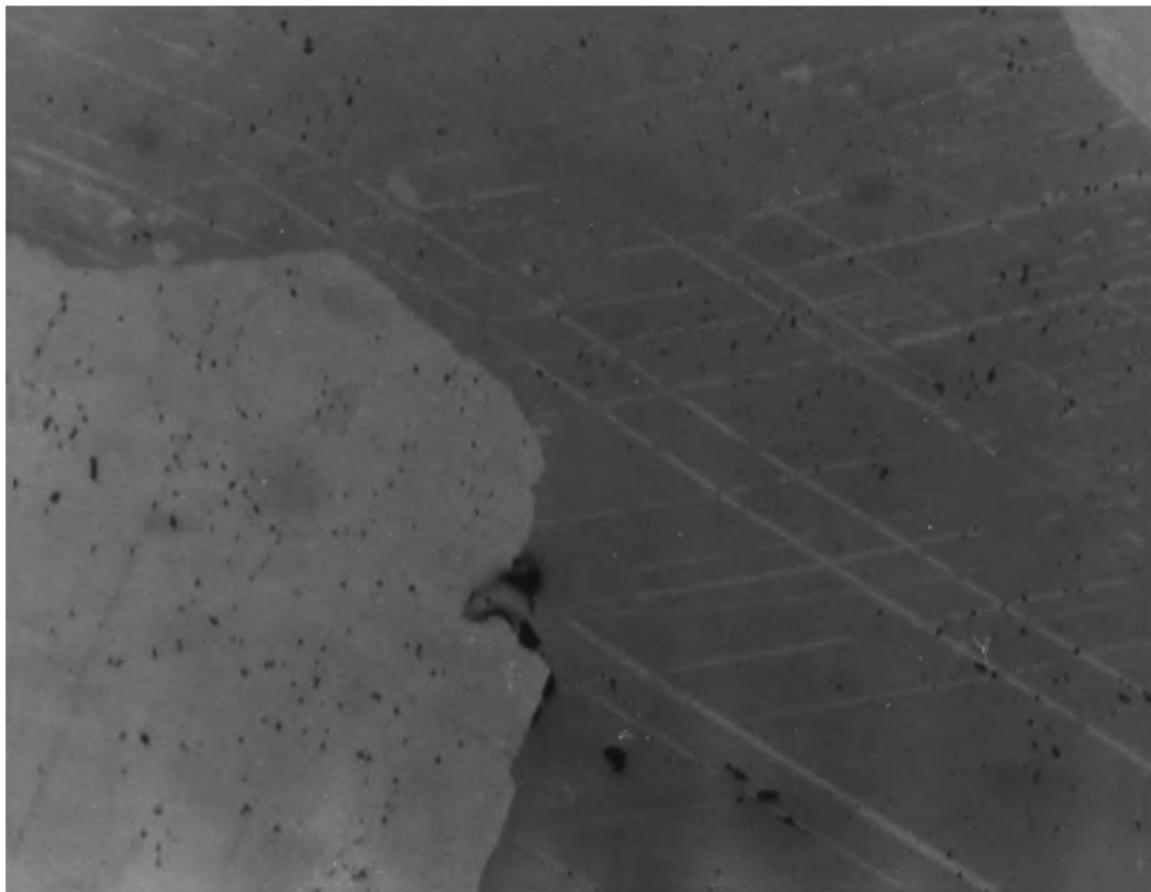
Plate 5.5.2a Calcite showing bireflection and lamellar twinning.
