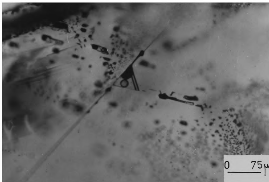
Plate 6.4.5b A primary fluid inclusion with a captive opaque mineral (in sphalerite).
