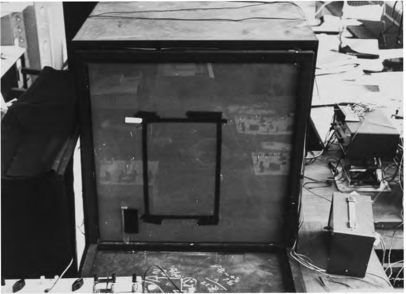
Figure 5.3 The rear projection screen as seen from the projectors.
