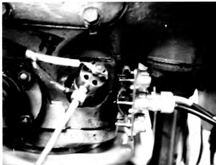
FIG. 4.1-2. The balanced-disc pressure pick-up (centre) shown mounted on the engine
