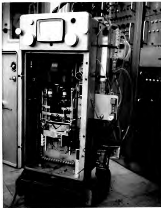
FIG. 9.2.3-2. The Luft and Grubb-Parsons analyser
