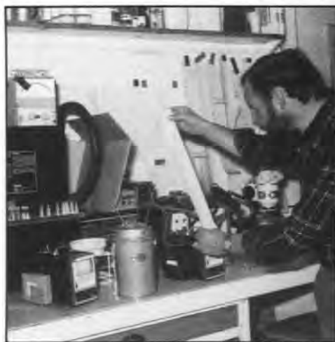
Figure 3. Reading the supercooling points of invertebrates from the chart record after a freezing experiment at the BAS station at Signy Island in the maritime Antarctic.
