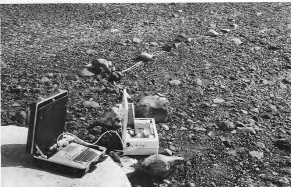
Fig. 1. Microclimate data logger (Grant Squirrel) located in a fellfield study area at Cape Bird, Ross Island. The Epson HX-20 microcomputer (in black case) is interfaced with the logger for data transmission.
