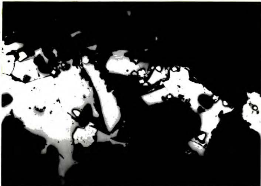
55. The second generation sphalerite (dark gray) and chalcopyrite relationship, Murgul mine. 160 x
