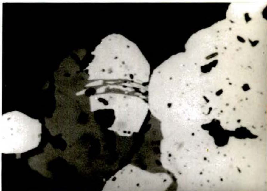
Pl. 31A. Shattered pyrite replaced by tennantite, ore Zone II closer to the ore Zone III. 600 x
