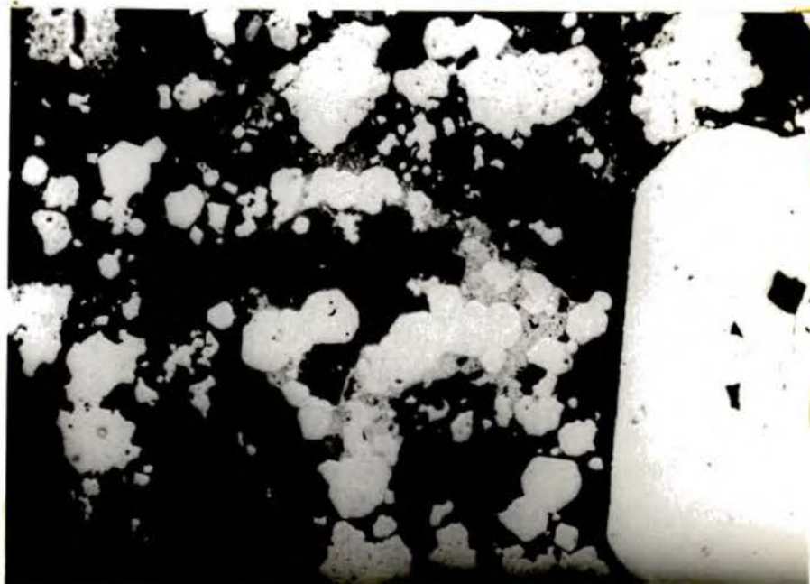
Pl.24. Colloidal pyrite-pyrite and sphalerite relationships, ore Zone II. 73 x
