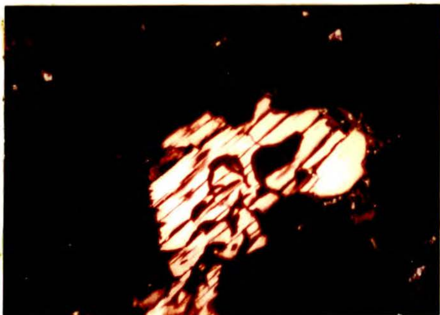
Pl. 34B. Covellite-bornite-pyrite relation, under cross nicols, ore Zone II, closer to the ore Zone I. 875 x
