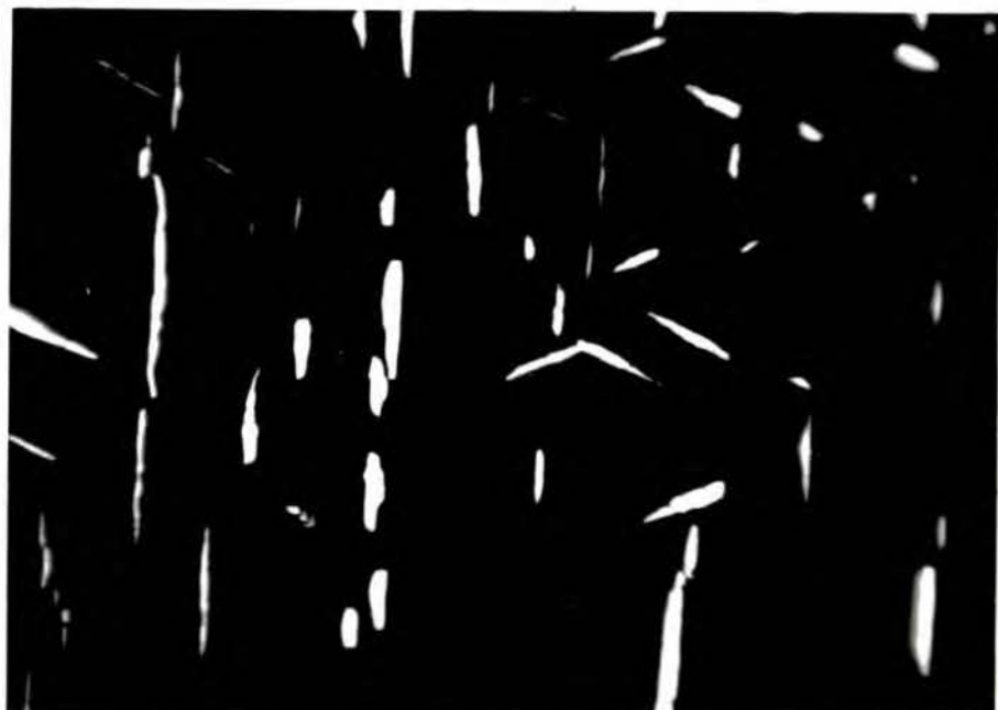
56. Chalcopyrite lamellae in sphalerite, Murgul mine. 2700 x
