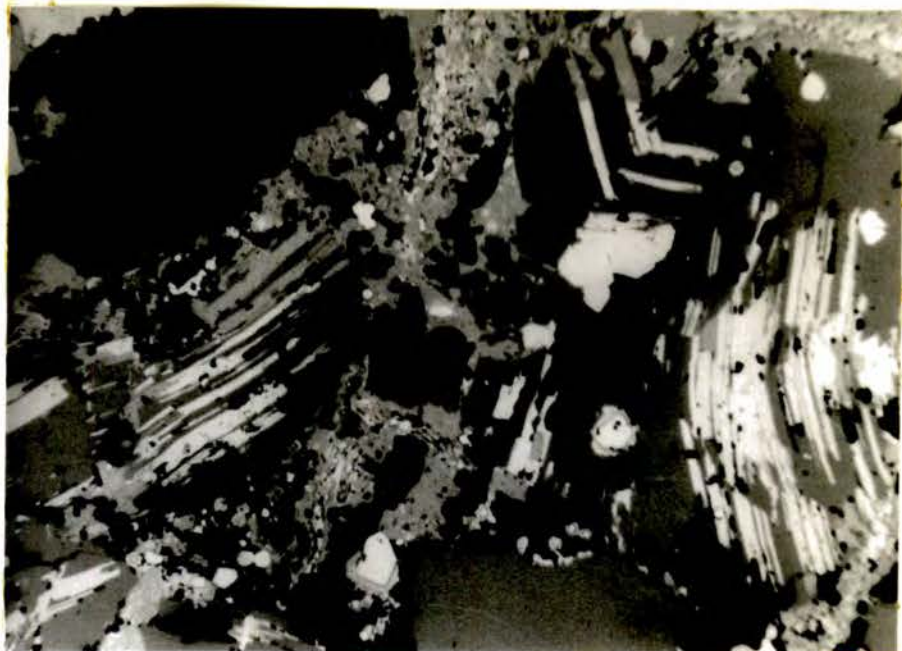
Pl.22. Guided replacement of sphalerite by chalcopyrite (whitish gray) and tennantite (gray), ore Zone II. 160 x
