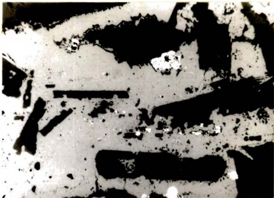
Pl. 20C. Sphalerite, gangue, barite relationships, ore Zone II. 160 x
