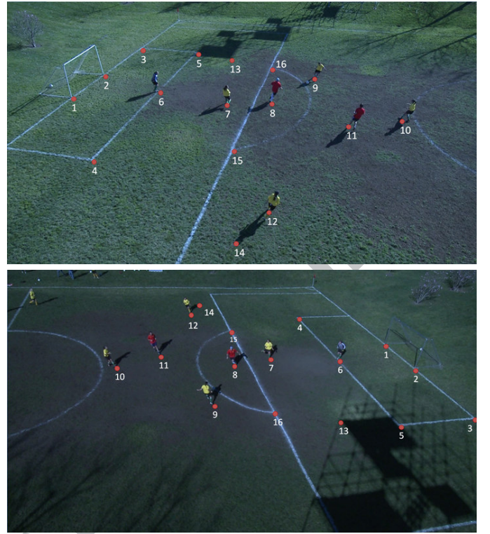
Fig. 8. Points on the image plane of the three cameras used to estimate the homography matrices between image planes 1 \leftarrow 2, 2 \leftarrow 3, and 3 \leftarrow 1. Note that all these points are co-planar. In practice, we found that the more spread out these points were, the better was our estimate of the homographies.
