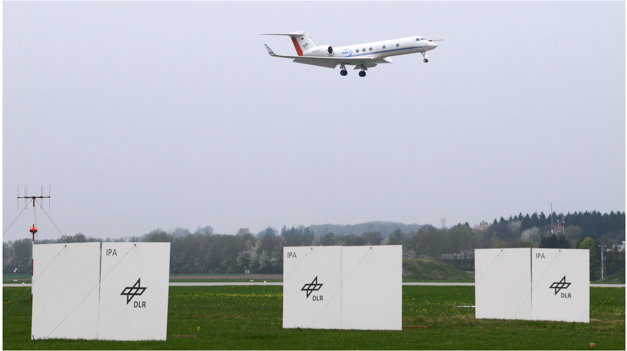
Abbildung 1.4.: Plate line consisting of six plates with dimensions 2.2\text{ m} \times 4\text{ m} displaced by 10\text{ m} designed for the dimensions of the HALO research aircraft (G550, photo Marc Malycha, DLR).
