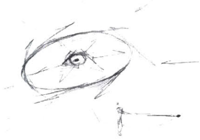
Summary of forces at work in orbital motion: centripetal force and acceleration inward, radially; centrifugal force outward, radially; tangential velocity.
