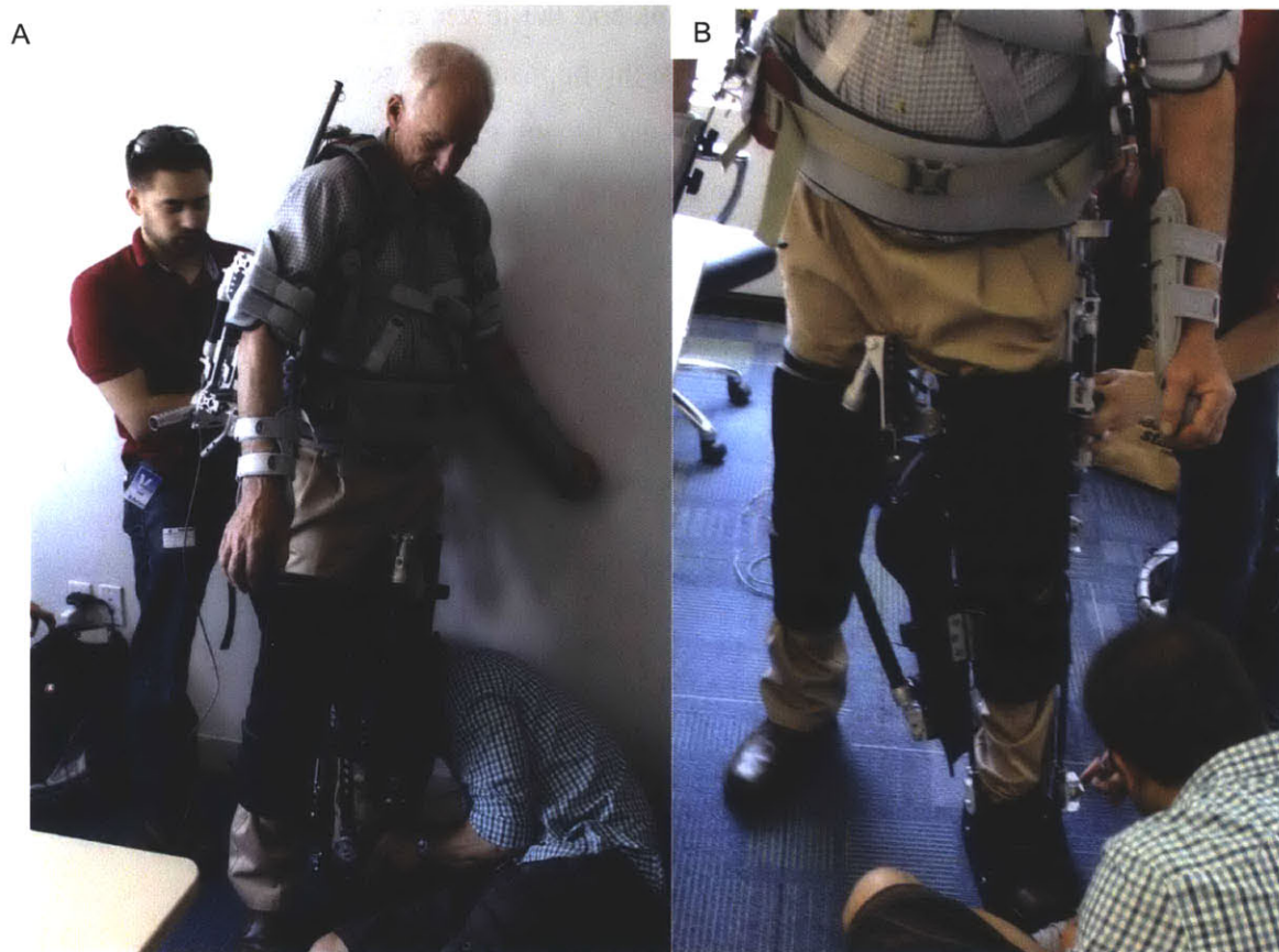
Figure 4.25 – Donning the EVA S3. (A) Adding the backpack. (B) Adjusting the knee and ankle assembly.
