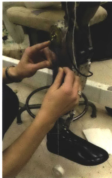
Figure 3.47 – Method for determining joint angle using a protractor and a plumb line
