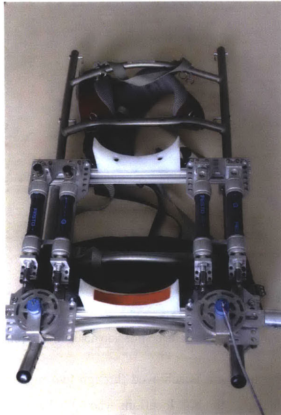
Figure 4.4 – The completed backpack with hip abduction/adduction actuator assemblies
