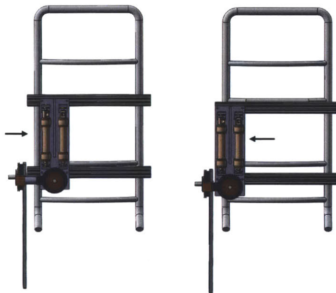
Figure 3.29 – Simplified model showing horizontal adjustment of hip abduction/adduction axis center
