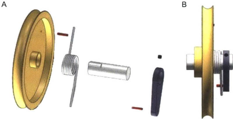
Figure 3.18 – Exploded view of retractable spool (A). Side view of Spool (B).
