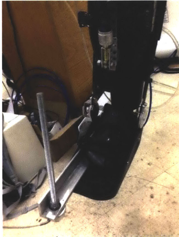
Figure 4.39 - View of ankle test setup. An L-bracket was used to manually move the ankle, since the RSST actuation was not working
