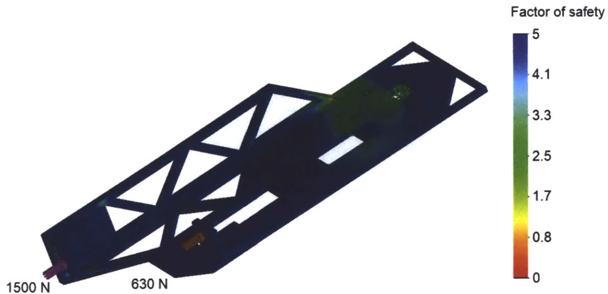
Figure 3.36 – Factor of safety FEA profile of a hip flexion/extension actuator assembly structure design iteration
