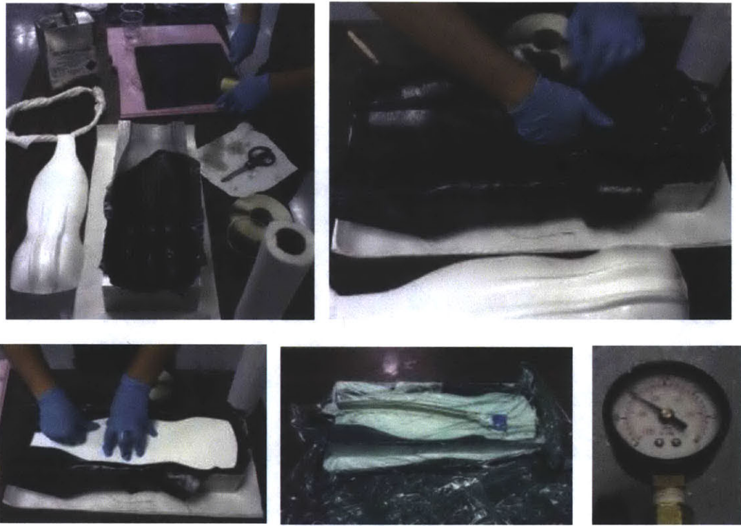
Figure 6.6: The carbon fiber greave layup process
