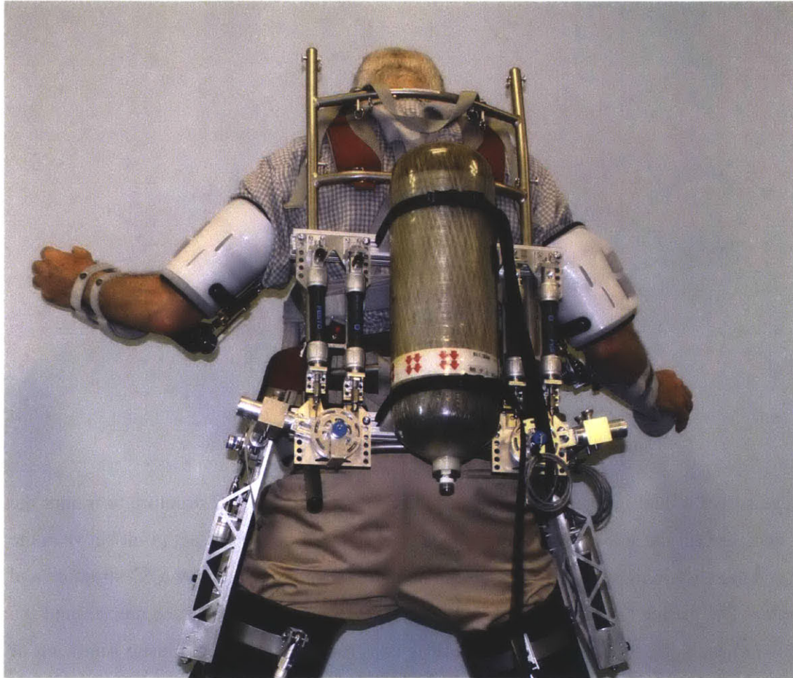
Figure 4.9 – Rear view of EVA S3 hip assembly on a subject.
