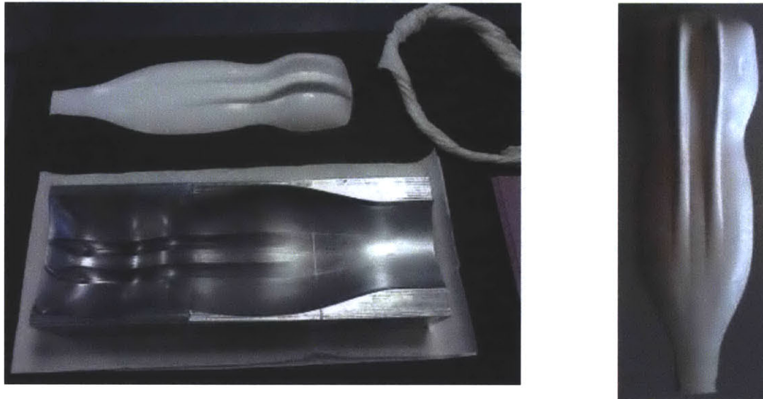
Figure 6.5: (A) Silicone plug with mold sections (B) Silicon plug for use during carbon fiber layups
