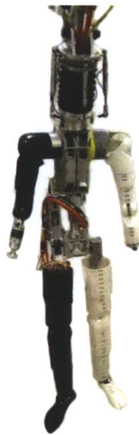
Figure 3.44 – The Robotic Space Suit Tester (RSST)
