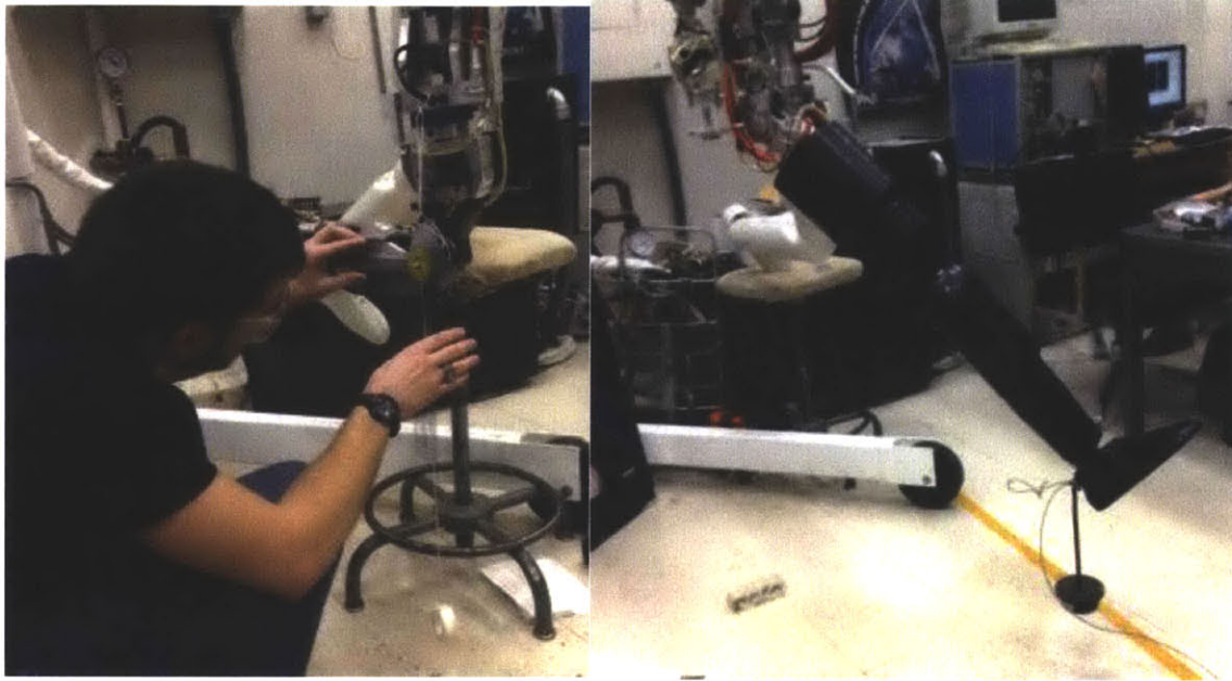
Figure 6.27 - Left: knee angle calibration (note protractor and plumb line). Right: hip flexion/extension torque calibration (note weight hanging from ankle).
