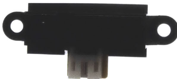
Figure 1-4: A Triangulation Based Distance Sensor : Sharp GP2Y0A21YK [5]
