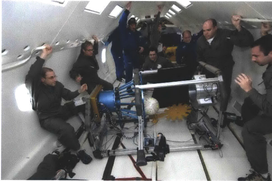
Figure 8: SPHERES-MOSR test bed performing OS contact dynamics experiments on reduced gravity flight
