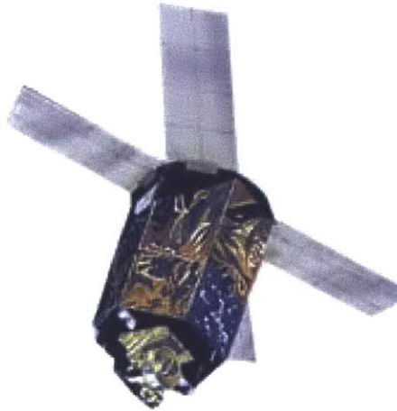
Figure 5-4: Shown above is GeoEye's OrbView-2 "SeaStar" satellite carrying the SeaWiFS ocean color sensor.
