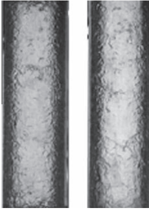
Fig. 8. Flow visualisation for annular flow G = 200 \text{ kg/m}^2/\text{s} and x = 0.20 : left in 1 - g, right in \mu - g.
