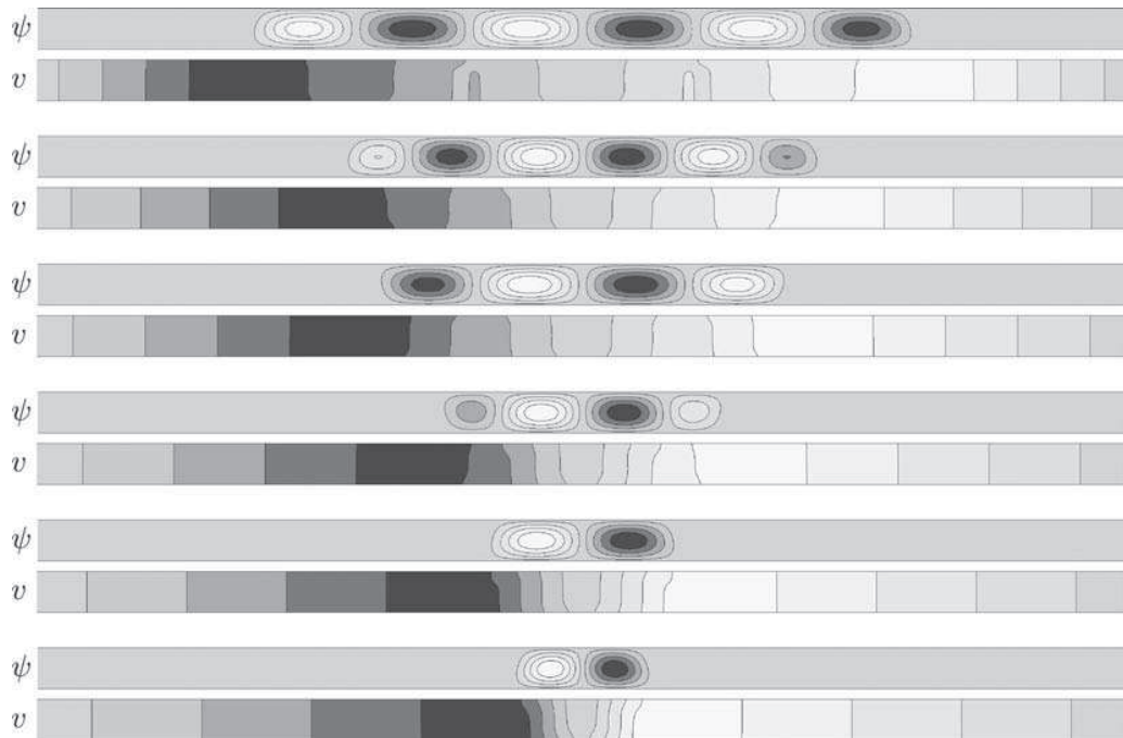
FIG. 2. Profiles of the L_{20}^+ solutions taken at the first 6 saddle-nodes from the diagram in Fig. 1, starting from the lower left. The solutions are represented using contours of the poloidal streamfunction \psi (upper panels) and the zonal velocity v (lower panels). The contour values differ from one solution to the next although the contours are in all cases equidistributed between their maximum and minimum values, black denoting positive values (clockwise motion) and white negative values (counterclockwise motion). Likewise black (white) indicates regions of positive (negative) zonal velocity v .
