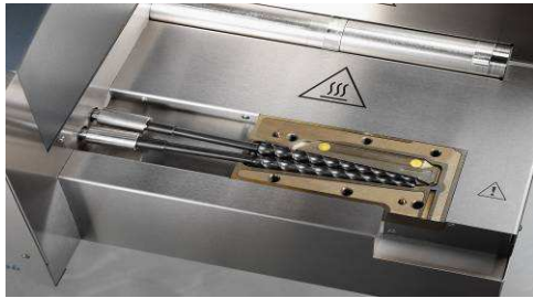
Figure 1 Configuration of the Minilab with the twin screws and the pressure transducers
