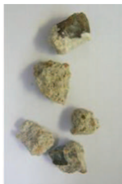
Unliberated aggregates, exhibiting various degrees of adhering cement paste.
