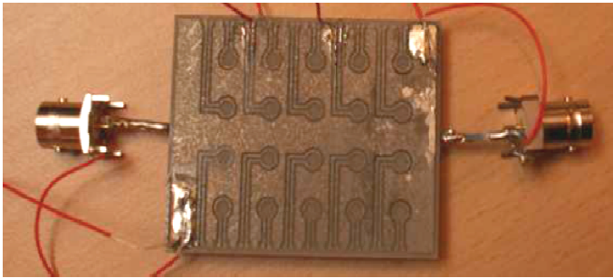
Fig. 15. View of EM-Matrix prototype #1: Ceramic substrate, diameter 3mm, BNC test connector.
