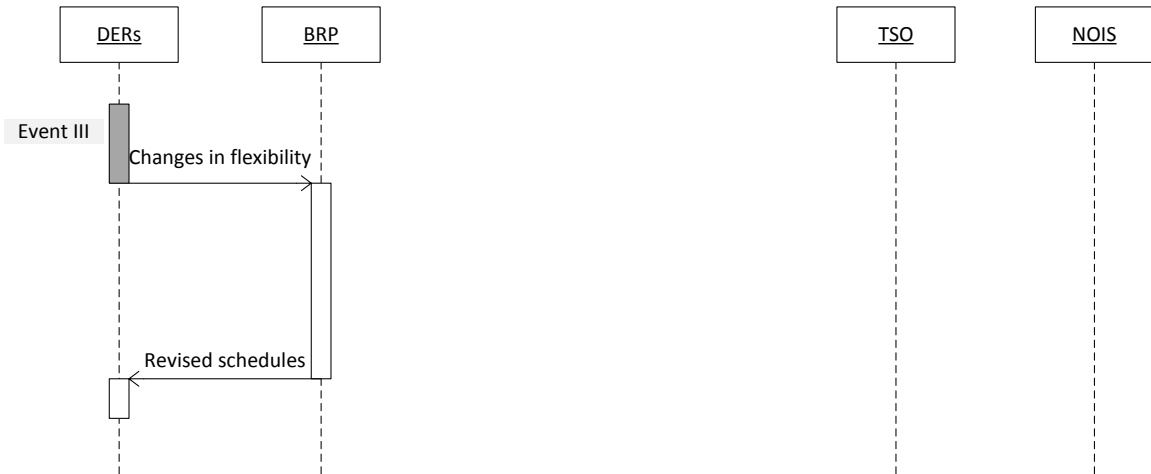
Figure 7 Alternative sequence showing communication in the Manual Regulating Power Market when one or more DERs experience small changes in their flexibility which does not require changing bids from the BRP, under direct control architecture.
