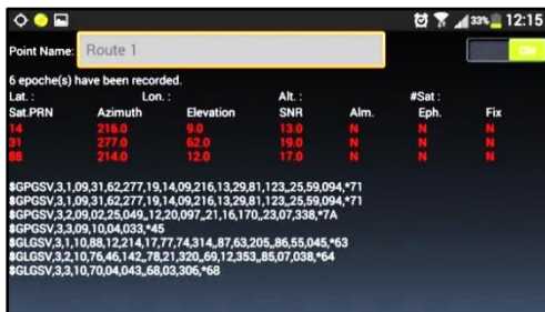
Figure 14 A screen shot of the developed Android app which is used to record GNSS data for shadow matching (including satellite PRN, signal-to-noise ratio, azimuth, elevation and conventional GNSS positioning solution).
